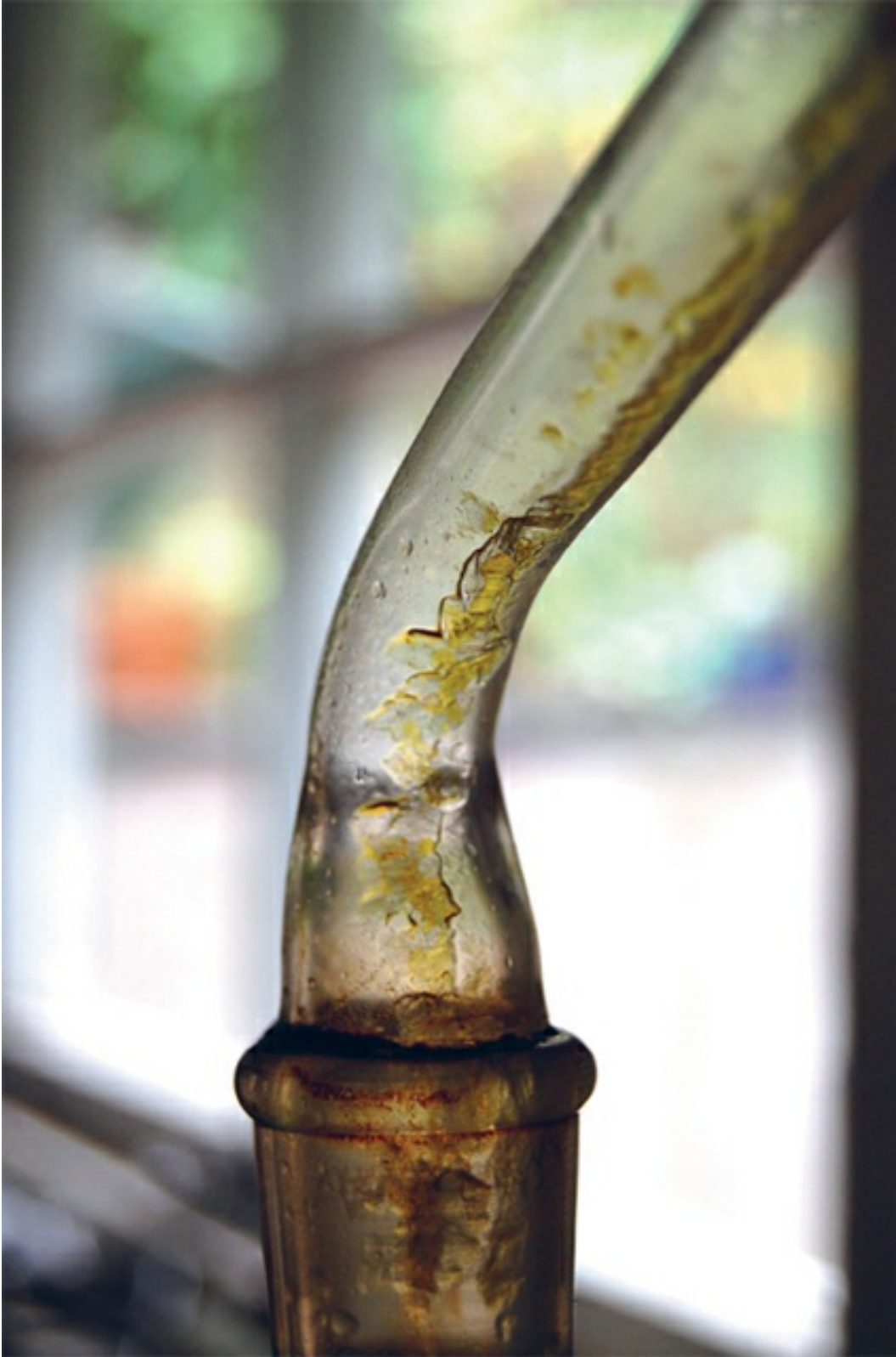
Sal ammoniac passing into the receiver
