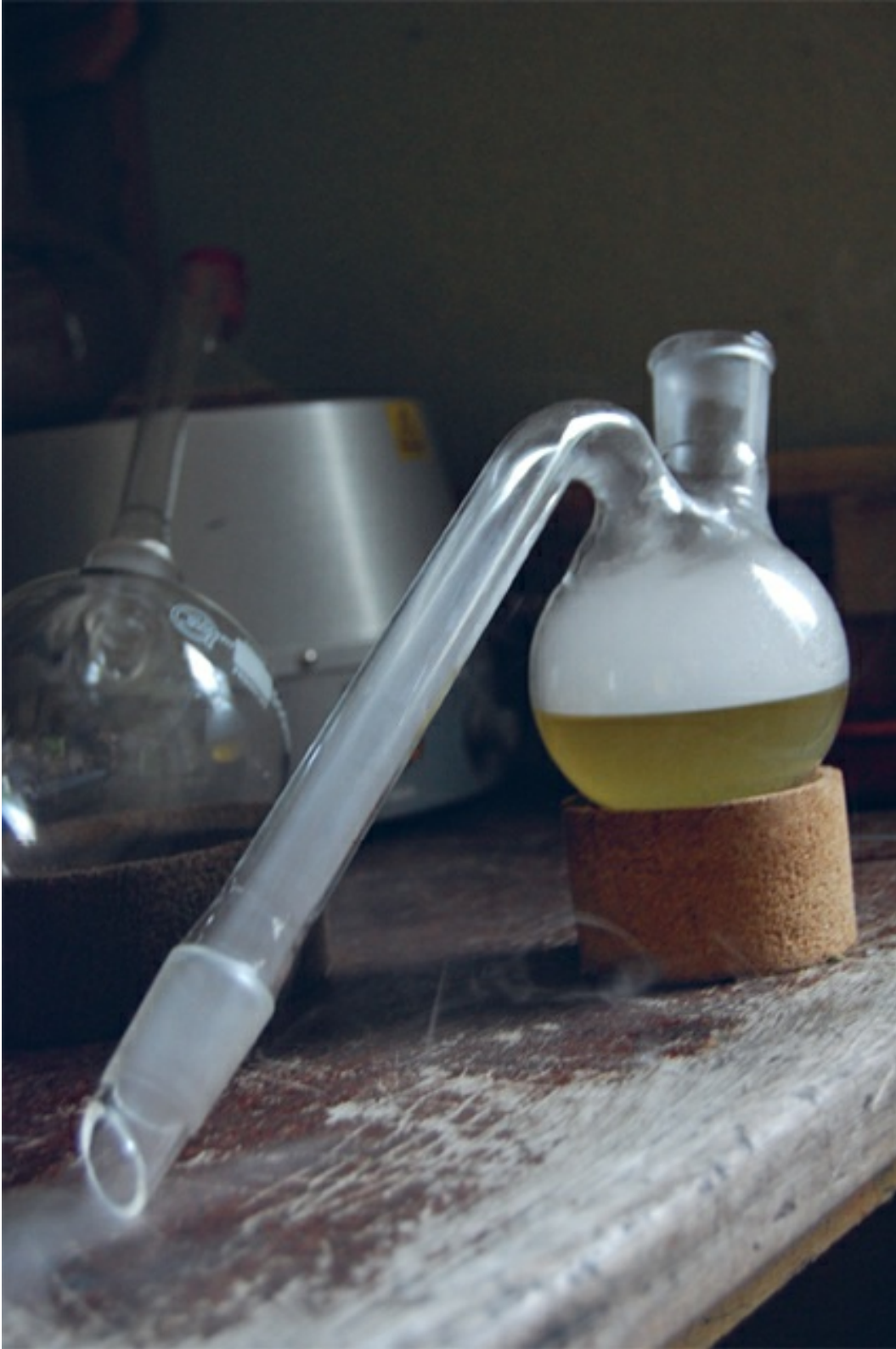
Seal the retort and distill
