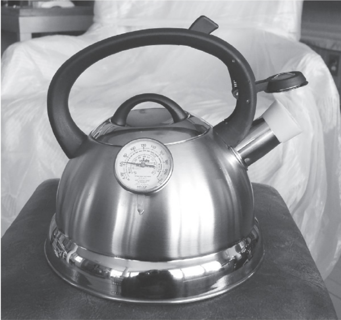
Fig. 5.3. Teakettle with thermometer installed and rubber stopper seated in spout.
