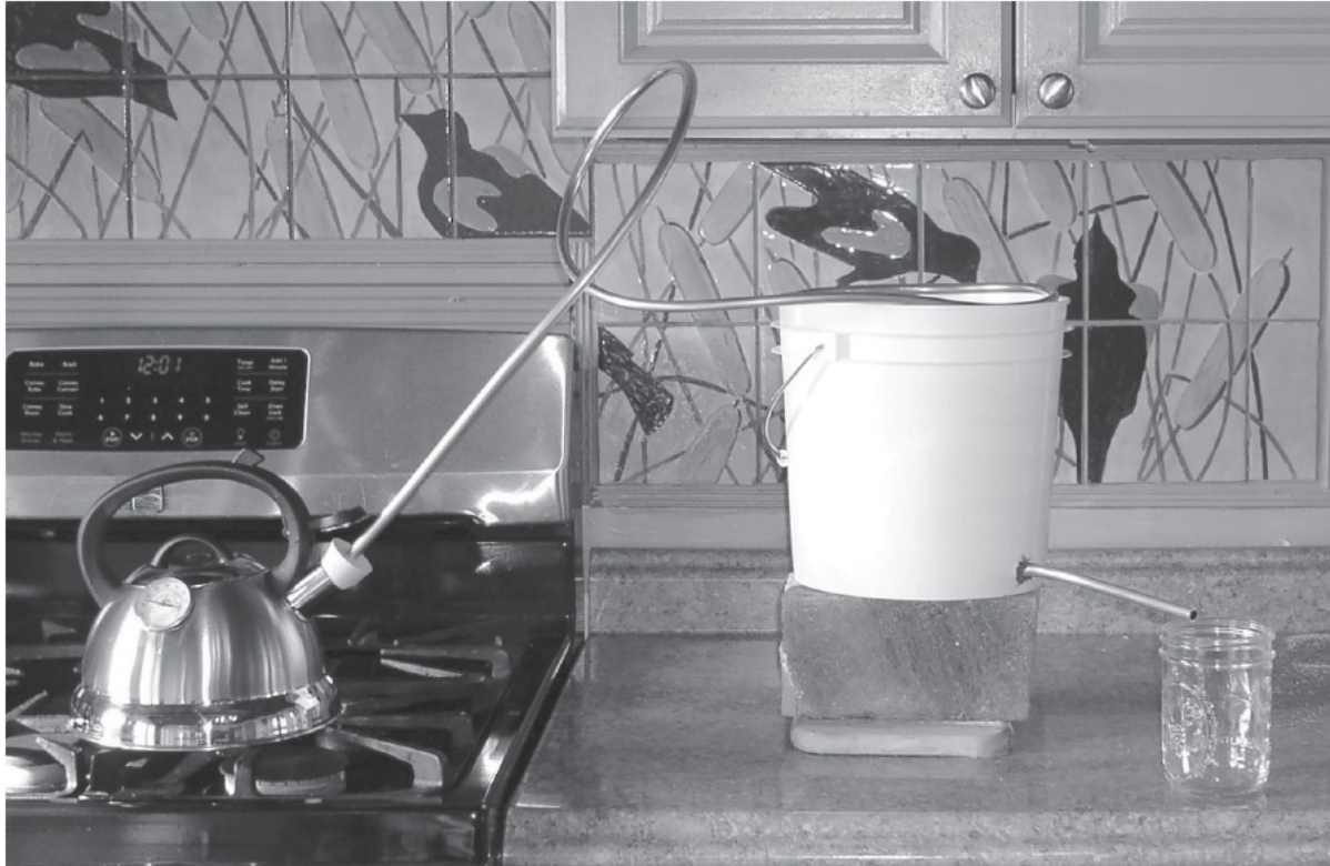
Fig. 5.4. Homemade alchemic still completed.
