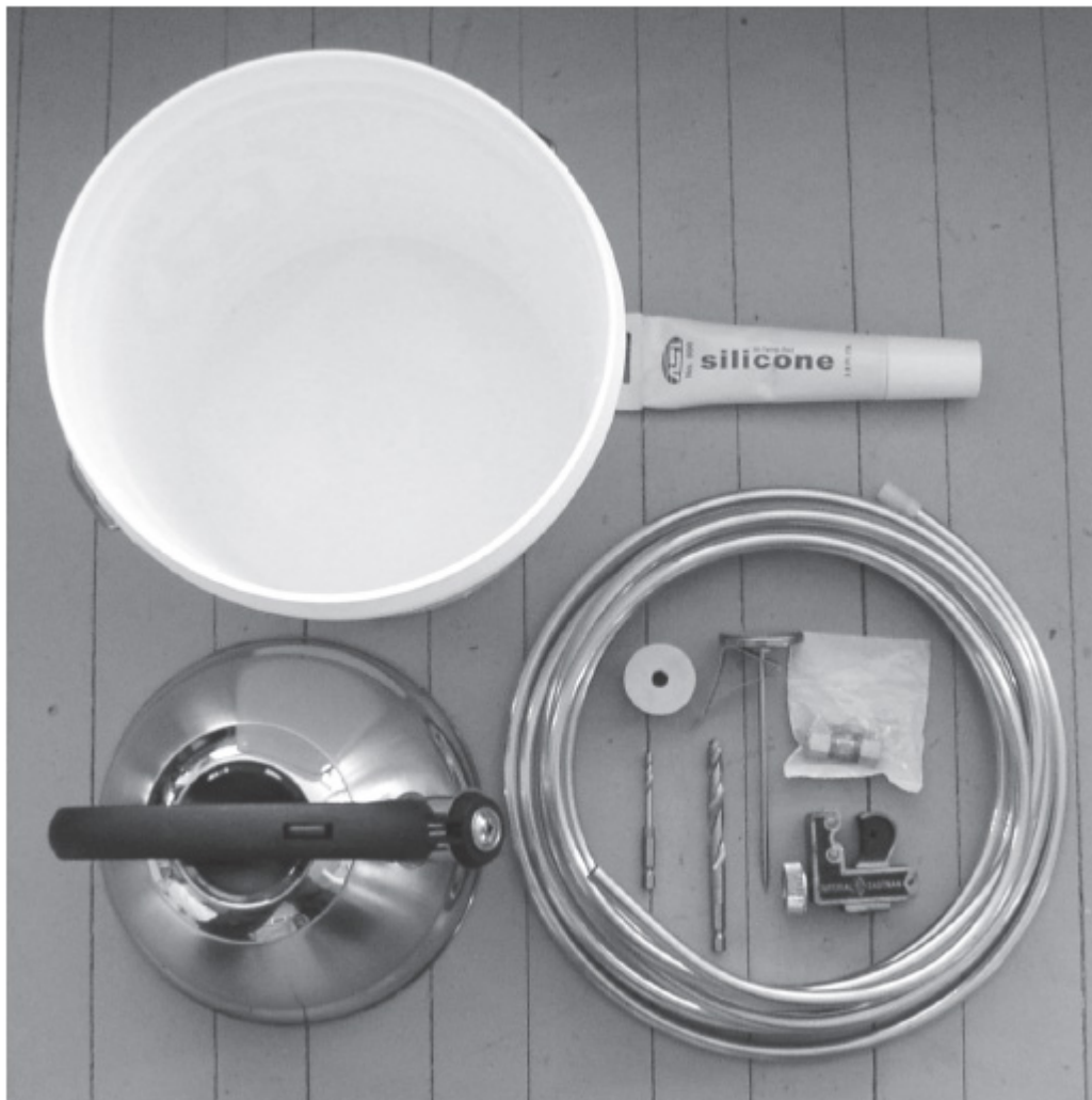
Fig. 5.1. Still fabrication supplies: bucket, silicone sealant, teakettle, copper coil, rubber stopper, thermometer, drill bits, tubing cutter.
