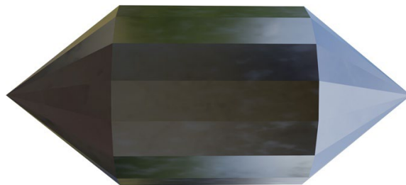
Fig 109 : - 16 SIDED END CONES ON A 16 SIDED CYLINDER CONSTRUCTION CUT-OUT
