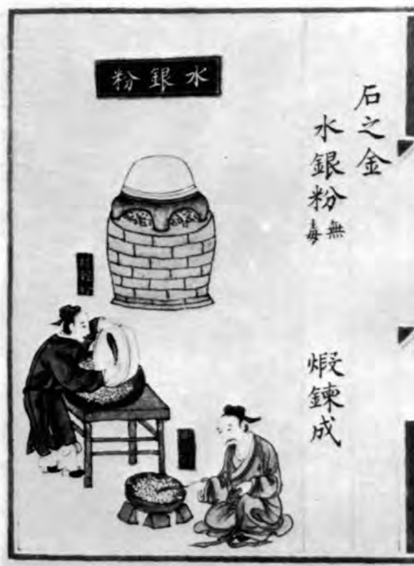
Fig. 1357. Sublimation of calomel, mercurous chloride, shui yin fên ; an illustration from a MS. copy of the Pên Tshao Phin Hui Ching Yao (+1505). Photo, Dr S. D. Sturton (1950), cf. Bertuccioli (1). This work (Essentials of the Pharmacopoeia ranked according to Nature and Efficacy) was edited by Liu Wên-Thai for the Imperial Library, and not printed at all until our own time. The picture comes from one of a family of MSS all having fine illustrations in colour, and preserved in various parts of the world.
