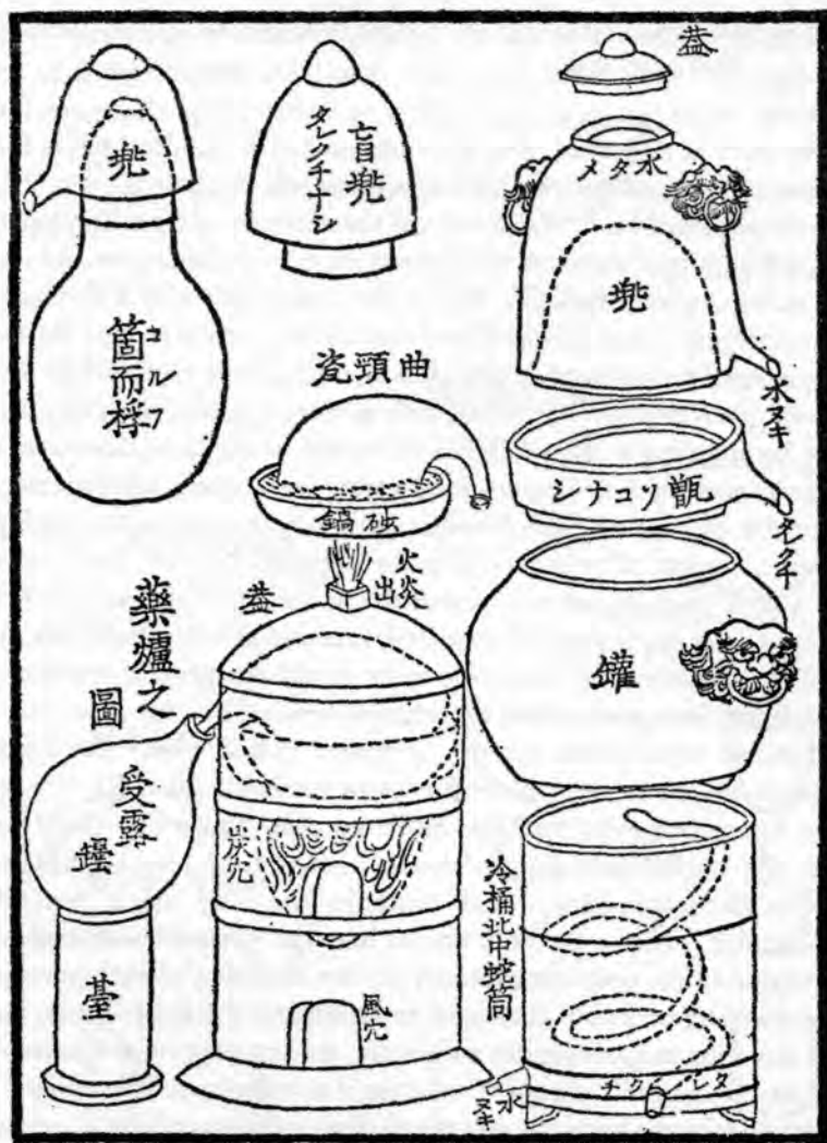
Fig. 1373. Some of the earliest illustrations of chemical apparatus in Japan, a page from the Ranka Naigai Sanbō Hōten (Handbook of the Three Aspects of Dutch Internal and External Medicine), published by Hashimoto Sōkichi in 1805. This was the entry of iatro-chemistry in a late phase of the Rangaku period. On the left at the top is an ambix with a helm, annular channel and side-tube; on the right a 'Moor's head' still in which the helm is water-cooled (cf. Vol. 5, pt. 4). On the left at the bottom is a retort protected in the furnace by a sand-bath, and with a receiver in position; on the right a cooling-coil condenser.
