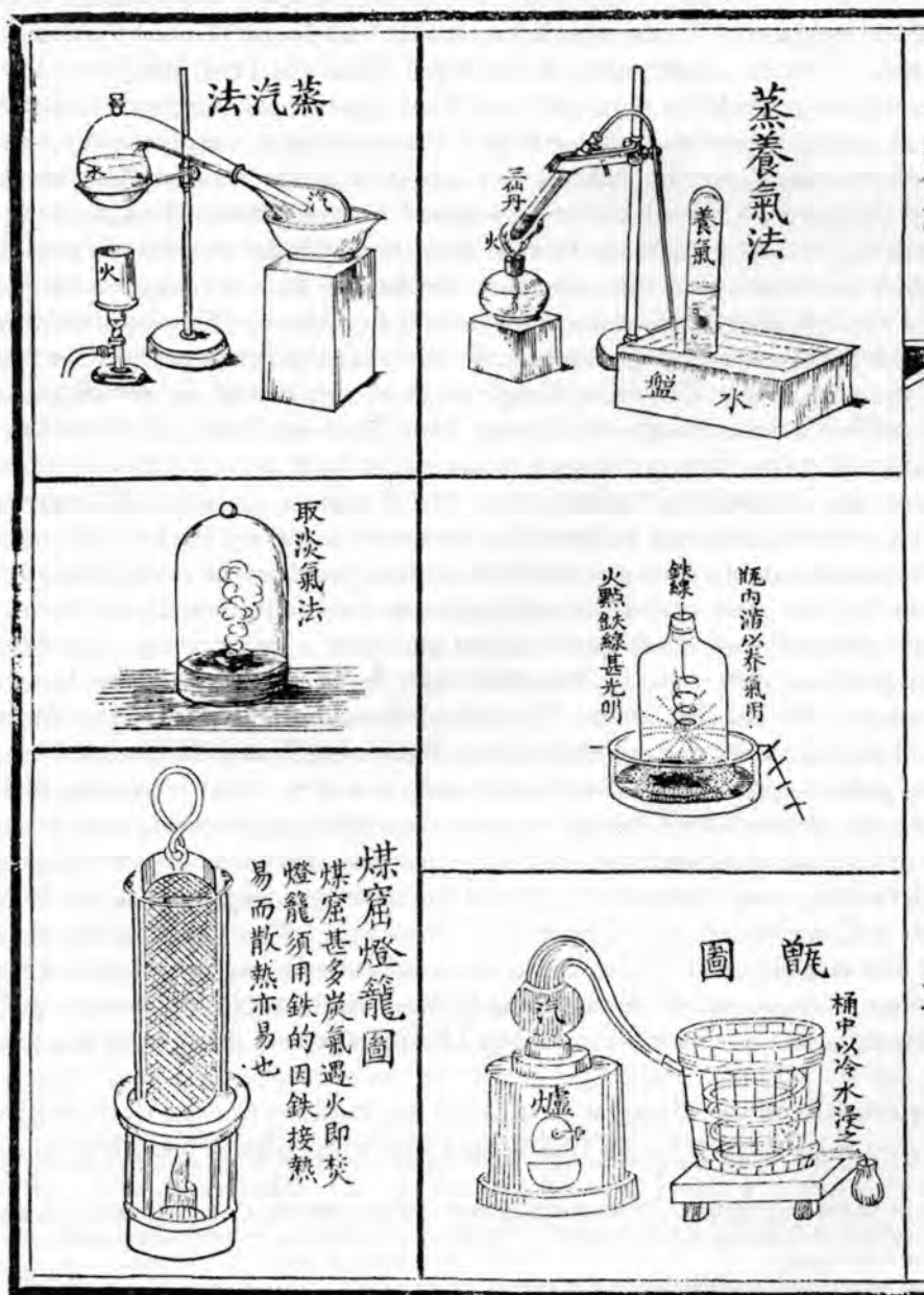
Fig. 1369. A page from the first book in Chinese dealing with modern chemistry, the Po Wu Hsin Phien , 1855 (New Treatise on Natural Philosophy and Natural History), written by an English physician, Benjamin Hobson (Ho Hsin, 1816 to 1873), then working in the hospitals of Canton and Shanghai. On the left one sees distillation with a retort, the preparation of nitrogen by heating ammonium dichromate, and Davy's lamp for miners. On the right oxygen is being collected over mercury, and a clean iron wire tipped with sulphur is burning vigorously in it, below, a distillation through a cooled coil is proceeding.
