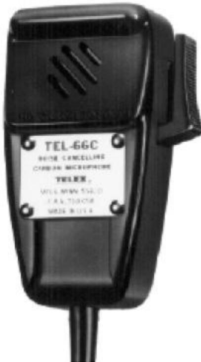
Figure 2-4. Carbon microphone
