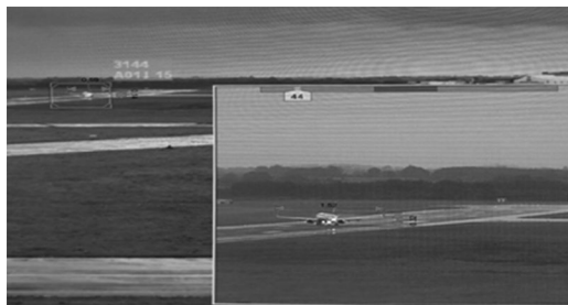
Figure 12.8 ATCO using PTZ camera to enlarge the visual perception to enhance situation awareness during B-737 landing.
