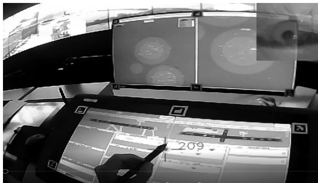
Figure 12.7 ATCO shifting attention from Shannon to Cork airport to pay attention on the runway activities on the EFS (fixation shown as red-cross recorded by eye tracker).
