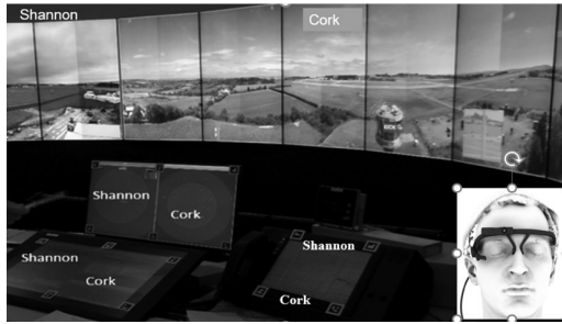
Figure 12.2 ATCOs using Pupil Pro Eye Tracker interacted with RTM comprised OTW, RDP, EFS and VCS (left-hand side are Shannon airport, right-hand side are Cork airport) for multiple remote tower operations.
