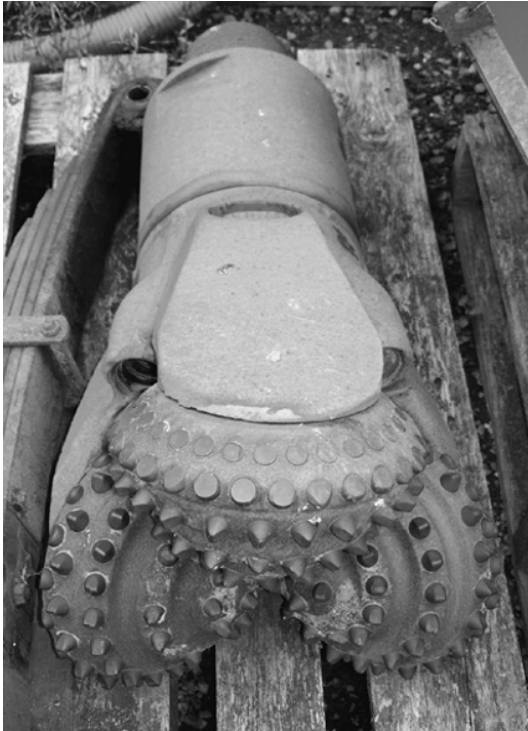
Figure 5.9 Rock-roller drill bit. Photo by Bruce Misstear
