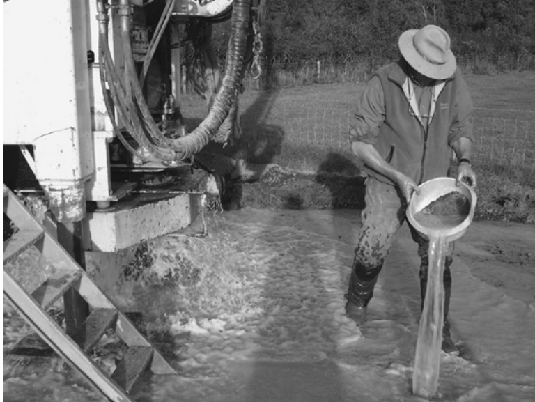
Figure 6.6 Hydrogeologist David Ball washing limestone drill cuttings collected during air rotary drilling (using a down-the-hole hammer), County Laois, Ireland. Photo by Bruce Misstear
