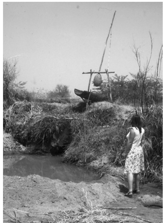
Figure 3.25 Shaduf used for lifting water from a temporary well in a dry river bed to an irrigated field beside the river bank, northern Nigeria. Photo by Bruce Misstear
