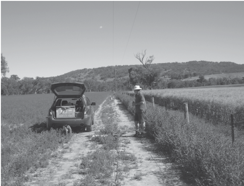
Figure 2.15 Electrical imaging near Wagga Wagga, New South Wales, Australia. Here the objective was to investigate the presence of saline groundwater. Photo (a) shows Bruce Misstear with the resistivity instrument (ABEM Terrameter), whilst photo (b) shows the line of electrodes and multicore cables (and colleague Ian Acworth). Photos by Ian Acworth (a) and Bruce Misstear (b)
