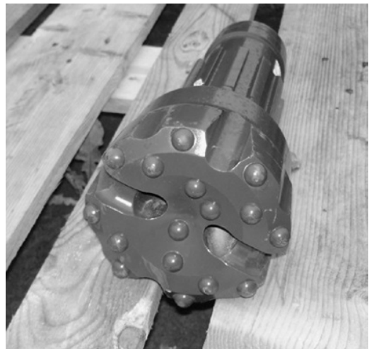
Figure 5.15 Button bit used for down-hole-hammer drilling. Photo by Bruce Misstear
