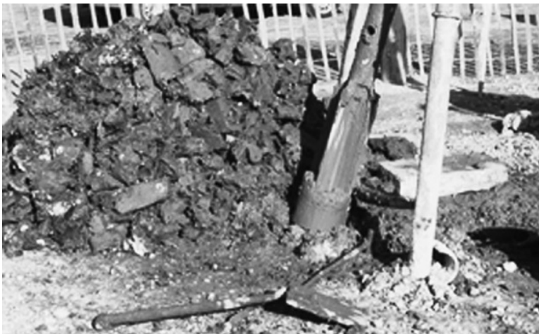
Figure 6.4 A clay cutter, used to extract samples of cohesive sediments encountered during cable-tool percussion drilling. Photo by Bruce Misstear
