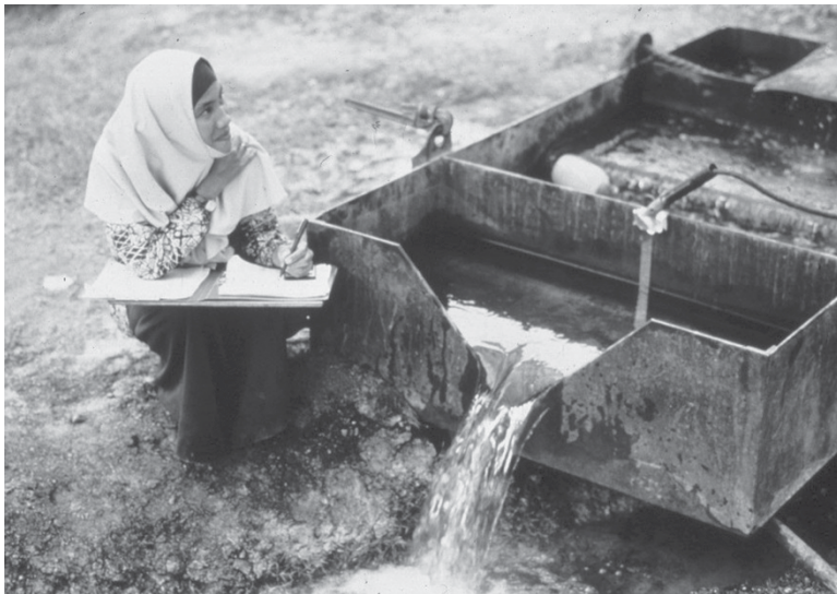
Figure 7.7 (a) The Norwegian hydrogeologist Steinar Skjeseth uses a watch and bucket of known capacity to determine the yield from a pumping test of a well. After Banks and Robins (2002) and reproduced by permission of Norges geologiske undersøkelse (Geological Survey of Norway). (b) A V-notch weir tank used during test-pumping in Malaysia. The height of water flowing over the weir can be related, with good accuracy, to the flow. The weir tank contains baffles to calm the discharge from the well. Photo reproduced by permission of David Ball
