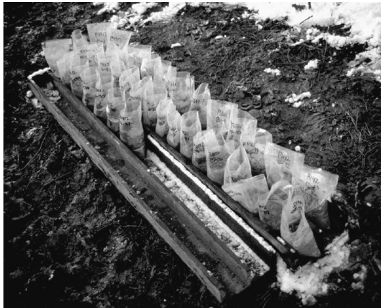
Figure 6.9 Disturbed formation samples placed in plastic bags. Photo by Bruce Misstear
