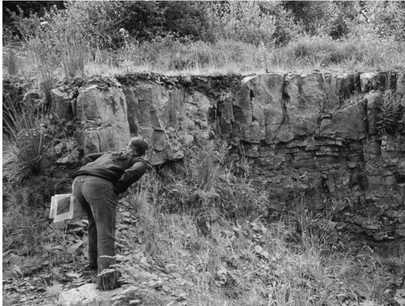
Figure 2.6 Examination of a quarry exposure of a fractured sandstone formation, County Monaghan, Ireland. Photo by Bruce Misstear
