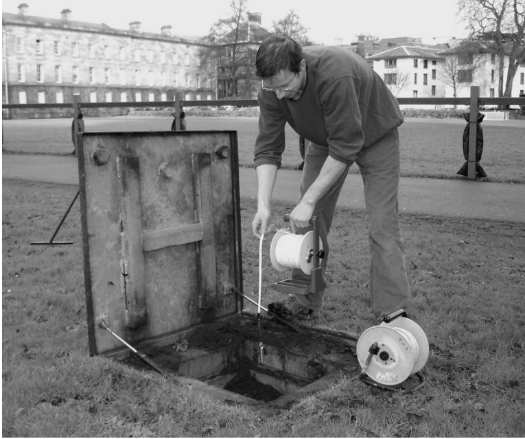
Figure 7.4 Measuring water level in an observation well in Dublin using electrical dipping tapes ('dippers'). Photo by Bruce Misstear
