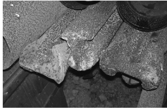
Figure 5.3 A rack of rather worn chisel bits used for percussion drilling. Photo by Bruce Misstear
