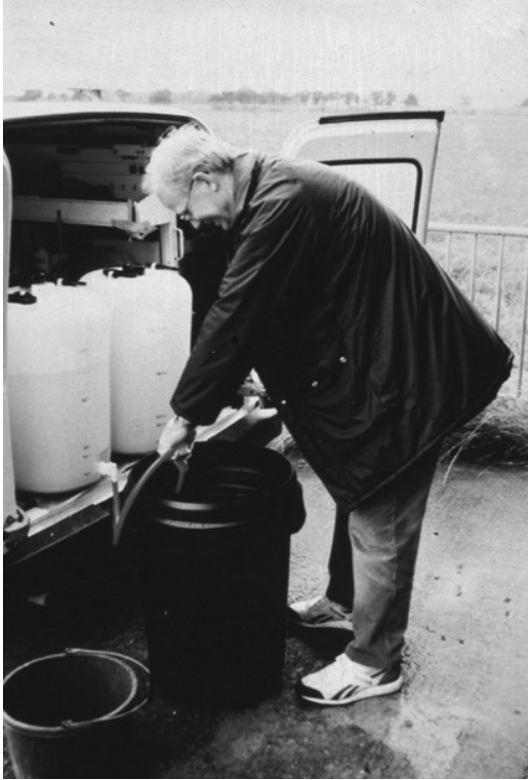
Figure 8.4 For some parameters, very large sample volumes are required. Here, Bruce Misstear prepares water samples for ^{14}\text{C} dating
