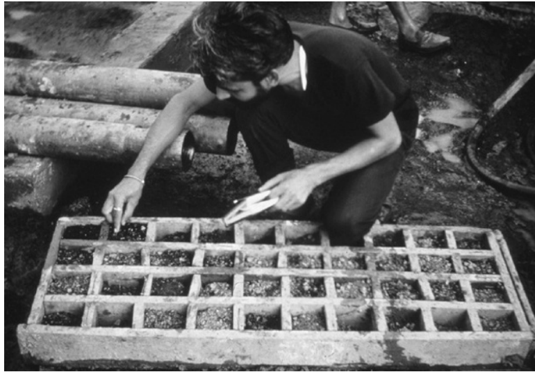
Figure 6.8 Disturbed formation samples being stored in sequential order of depth on site in a compartmentalized sample box. Reproduced by permission of Paul Ashley, Mott MacDonald Ltd
