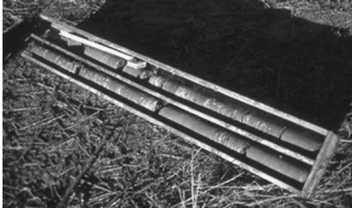
Figure 6.13 Storage of newly extracted cores in a core-box, landfill site, England. Photo by Bruce Mistear
