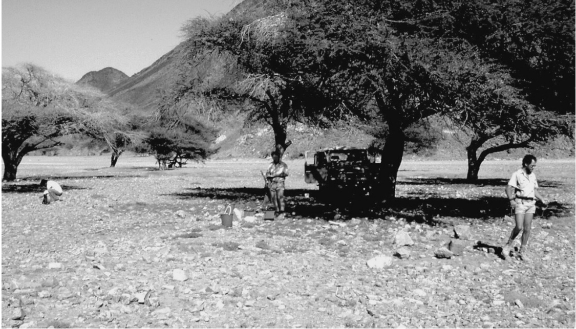
Figure 2.13 Vertical electrical sounding in the Red Sea hills region of northern Sudan. The objective here was to identify the thickness of wadi gravel aquifer overlying low permeability volcanic bedrock. The resistivity instrument and operator are in the centre of the picture, partly shaded by the tree, whilst the person on the left is connecting a cable drum to one of the electrodes. The bucket of water (just to the left of the resistivity instrument) was used to water the contact point between each electrode and the ground surface in this very arid region. Photo by Bruce Misstear
