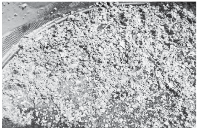
Figure 6.5 (a) Direct circulation rotary drilling in Faryab Province, Northern Afghanistan. Samples of alluvial sand and gravel were collected in a sieve (c) from the drilling mud and then stored in flasks clearly labelled with depth intervals (b). Fine material may be under-represented in the samples. (a)–(c) reproduced by permission of NORPLAN, Norway
