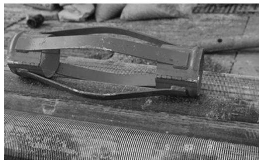
Figure 5.19 Casing centralizer (lying on top of two lengths of wirewound screen). Photo by Bruce Misstear
