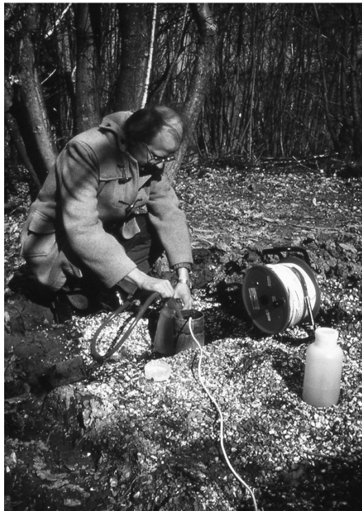
Figure 8.9 (a) David Banks uses a narrow-diameter electric submersible pump to sample a monitoring borehole near a landfill at Trandum, Norway. The pump is powered by a small portable generator and its speed is controlled by a frequency regulator. (b) Bruce Misstear uses a tiny, low-cost submersible pump (of the kind employed as a bilge pump in boats) to sample an observation borehole near a landfill in southern England. The pump is powered from a 12 V car battery
