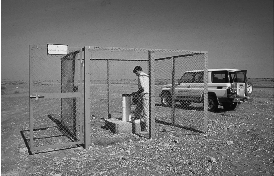
Figure 3.13 An observation borehole located near to an artificial recharge dam in northern Oman. Photo by Bruce Misstear
