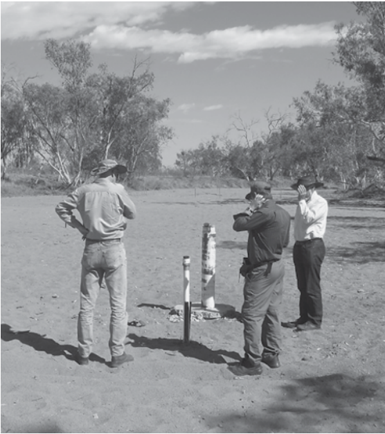
Figure 3.16 Borehole clusters: (a) small diameter observation boreholes installed to different depths in dry river bed near Alice Springs, Australia, (b) cluster of larger diameter boreholes constructed in glacial overburden and crystalline rock aquifers in County Donegal, Ireland. Here, larger completion diameters were chosen to enable pumping tests to be carried out in the boreholes. Photos by Bruce Misteear
