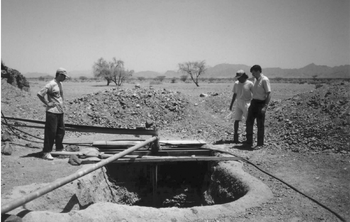
Figure 2.9 Examining a hand-dug well in northern Oman. The well is fitted with a belt-drive turbine pump. Note the excavated spoil material piled up behind the well, which can give a useful indication of the well geology. Photo by Bruce Misstear
