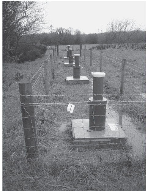
Figure 3.16 Borehole clusters: (a) small diameter observation boreholes installed to different depths in dry river bed near Alice Springs, Australia, (b) cluster of larger diameter boreholes constructed in glacial overburden and crystalline rock aquifers in County Donegal, Ireland. Here, larger completion diameters were chosen to enable pumping tests to be carried out in the boreholes. Photos by Bruce Misteear
