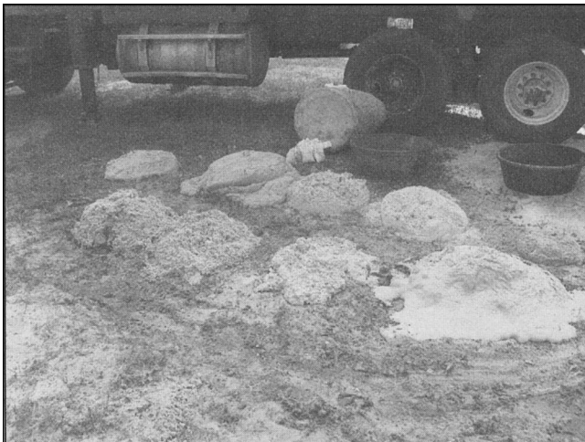
Figure 3-27 Sample from cyclone on typical reverse-air, dual-tube drill rig
