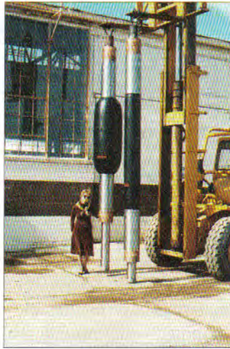
Figure 10.23. Inflatable packers are used as permanent or temporary sealing devices to isolate portions of the wellbore (Baski Inc.).
