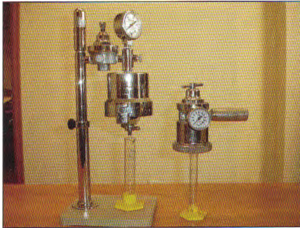
Figure 8.10. A filter press (e.g., full-area press left side, half-area press right side) can be used to measure the flow rate of water through a specific thickness of filter cake (Quality Drilling Fluids).
