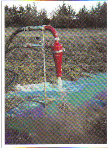
Figure 8.20. A correctly adjusted desander in a properly maintained system has a fan-like discharge with minimal entrained solids (© 2005 Baroid, a Halliburton PSL).
