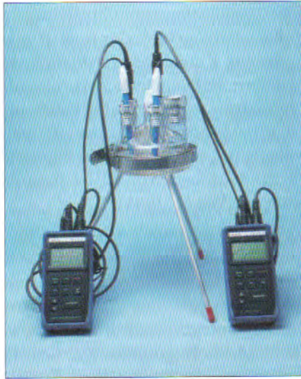
Figure 5.4. A flow-through cell measuring specific conductivity, pH, Eh, and dissolved oxygen.
