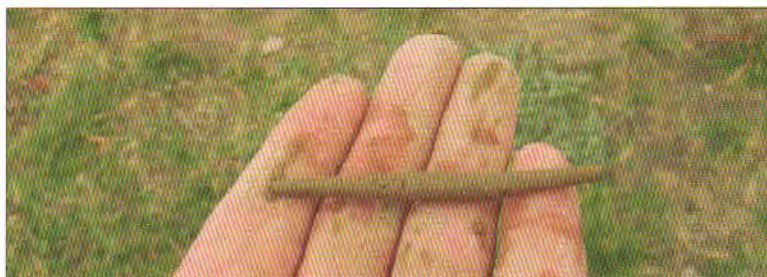
Figure 3.15. Clays can be rolled into ropes ¼-in (6 mm) in diameter; silts cannot be rolled into ropes.
