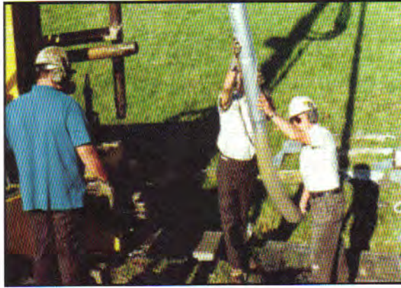
Figure 3.4. Core sample being collected using sonic drilling (Sonic Drilling Ltd.).
