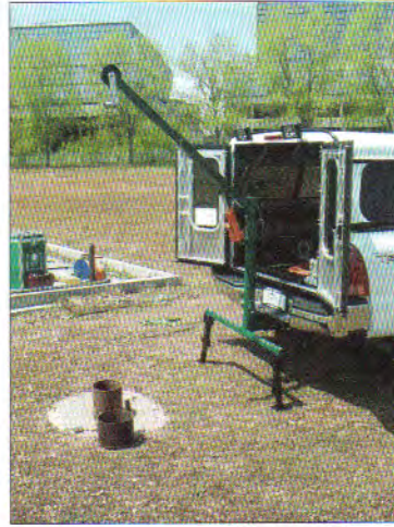
Figure 4.4. Typical small-truck groundwater-logging system (Mount Sopris Instruments).
