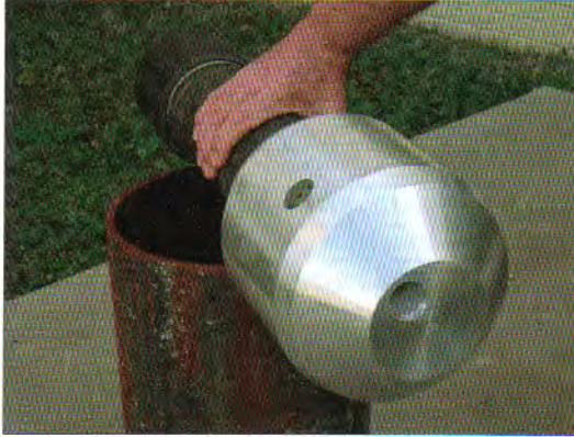
Figure 11.10. The Baski BJT-8, 8-in (200-mm) jetting tool (made for 10-in (250-mm) wells) has 4 jets that are diametrically opposed and 1 bottom jet (Baski, Inc.).
