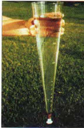
Figure 11.21. An Imhoff cone is used to estimate sediment concentration, but the small volume of the cone limits its accuracy.
