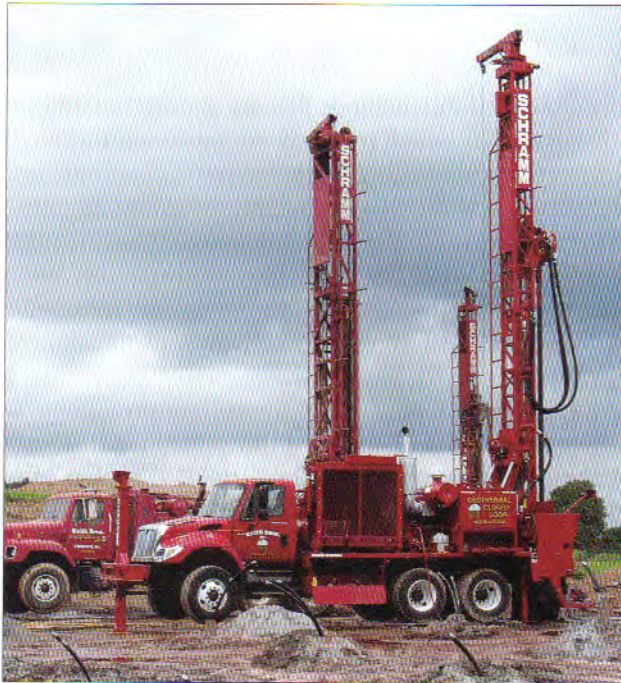
Figure 7.1. Tophead drilling rig (Schramm, Inc.).
