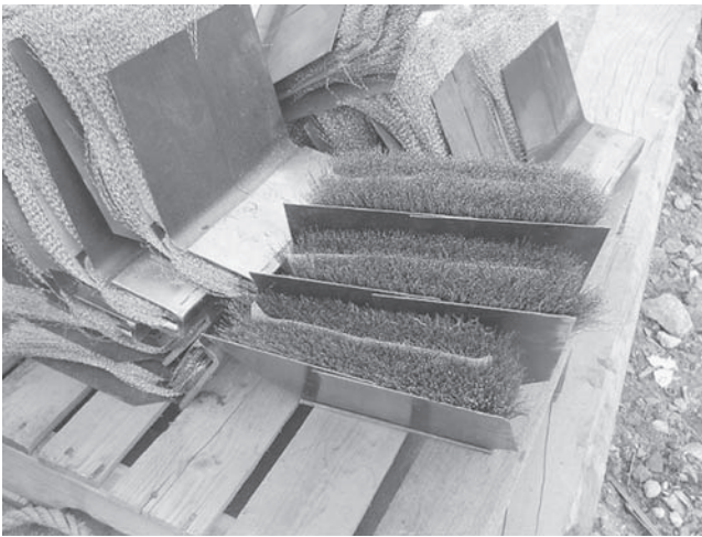
Figure 4.13 Wire Brushes for Tail Seal
