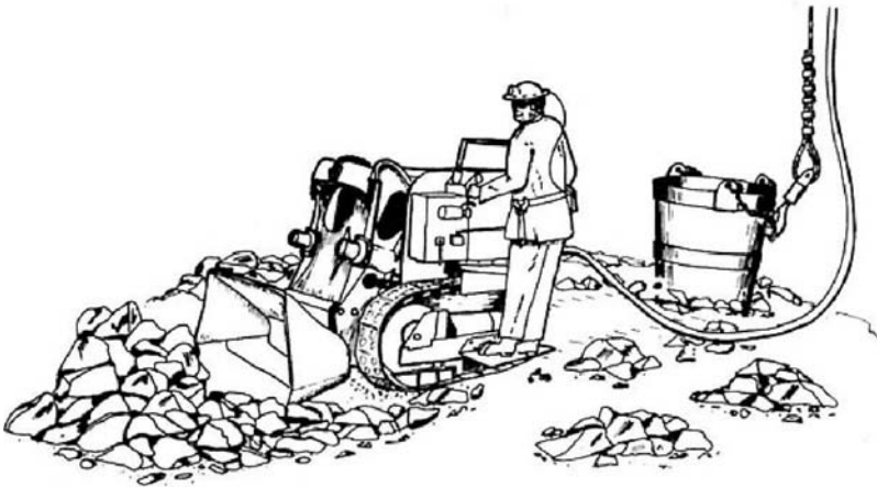
Figure 9.1 Eimco 630 Overshot Rail-Mounted Mucker (Courtesy of the Society for Mining, Metallurgy, and Exploration)
