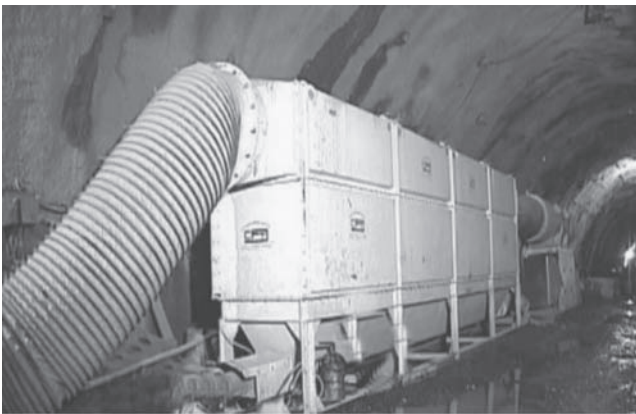
Figure 6.5 Roadheader Dust Collection System
