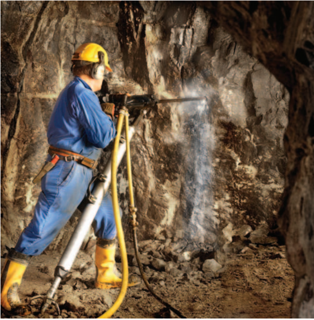
Figure 5.2 Photograph of Jackleg (Photo: Atlas Copco)
