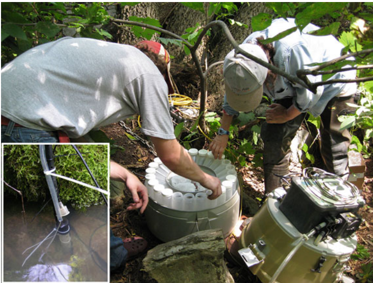
Fig. 4 Automatic ISCO stormwater sampler with 24 1-L bottles used to collect stormwater discharge at the springs. Inset shows water level trigger and pump tubing intake
