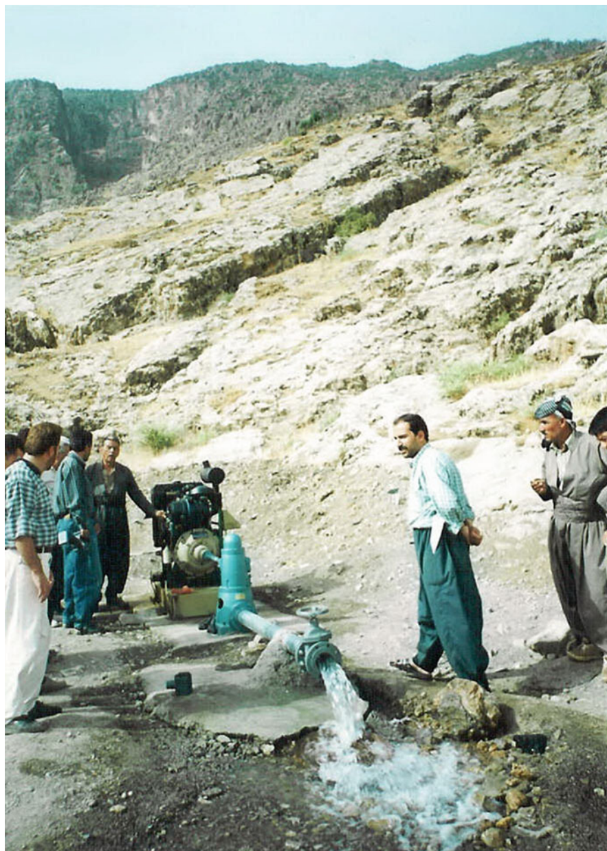
Fig. 15 One of the wells drilled in the Bekhme aquifer for the purpose of irrigating orchards affected by drought (Shaqlawa, northern Iraq)
