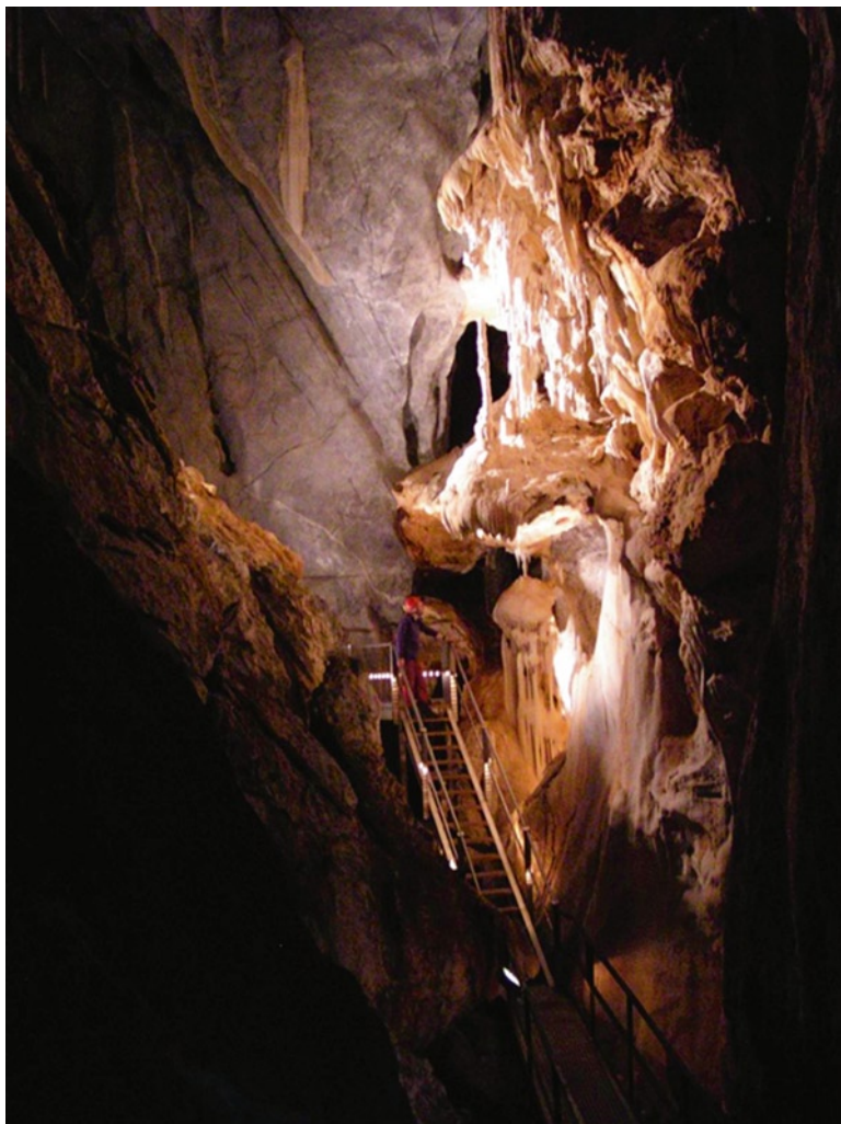
Fig. 6.5 Re-lighting of the Donna Cave, Chillagoe Queensland. Main lighting sequence is controlled by c-bus programming and can be modified by a guide. Tracklights are low energy use LEDs. Note use of inert materials – plastics and stainless steel – for all stairs and railings (Photo by David Gillieson)
