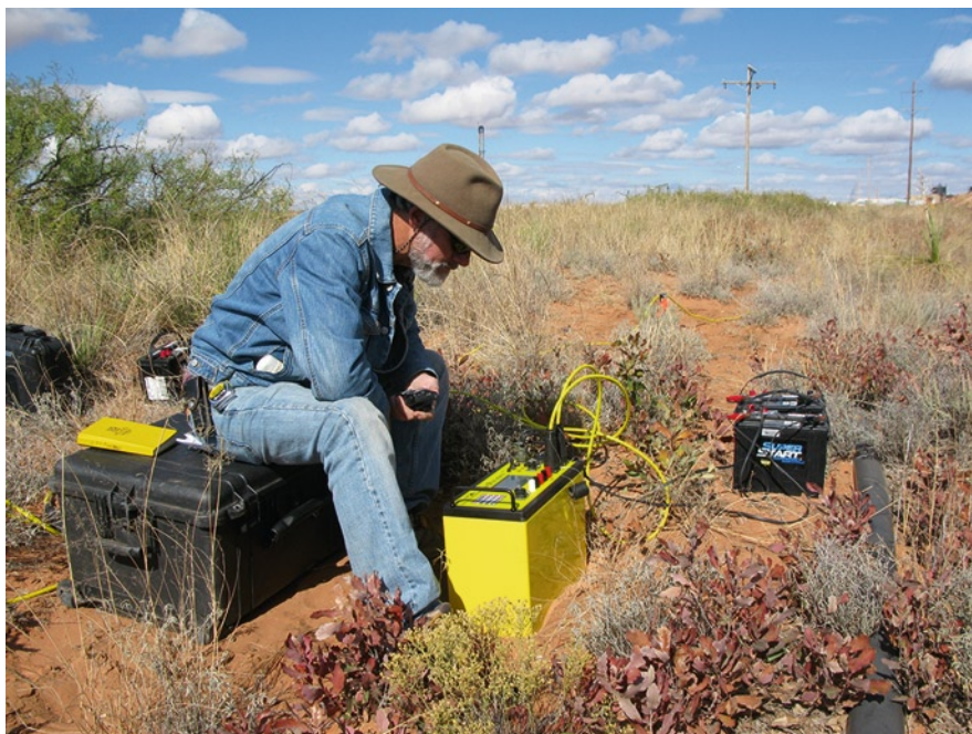
Fig. 14.5 NCKRI conducts geophysical surveys to map subsurface karst hydrogeology and to evaluate the potential for collapse or subsidence
