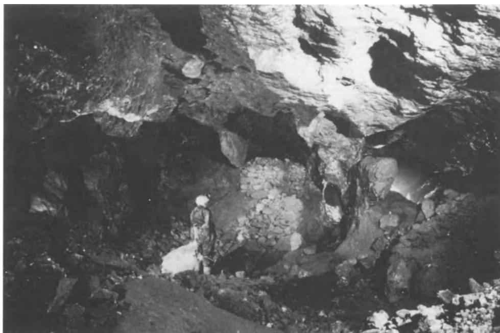
Figure 4.17 Ribs of limestone left around solution cavities which were filled and then re-excavated by miners in the Black Ox Mine workings in Great Masson Cavern. (Photo: T.D. Ford.)
