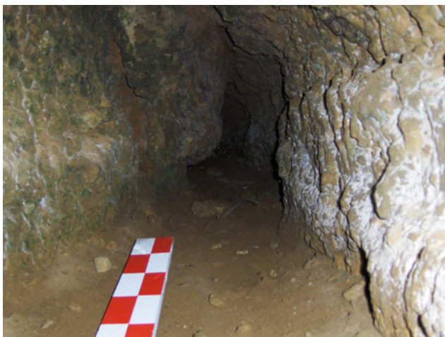
Fig. 7.5 View looking west into the Mosquito Cave. This is what most of the passages or drifts in the Dubuque area look like after miners removed the sediment. At this point it is roughly three quarters meter wide and one meter tall. The white material is tentatively identified as goslarite ( \text{ZnSO}_4 \cdot 7\text{H}_2\text{O} ) Scale bar divided into 0.1 m units
