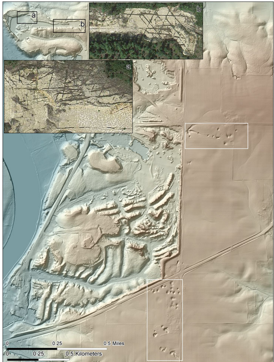
Fig. 5.32 Shaded relief lidar showing two groups of cover-collapse sinkholes overlying Ordovician-age Galena–Platteville limestone near Dixon in Lee County. This represents the North-Central karst area, where glacial till is relatively thin. Lidar data provided by the Illinois Height Modernization Program (clearinghouse.isgs.illinois.edu) supported by the Illinois Department of Transportation. The linear features within the quarry (a, b) are due to vegetation growing along crevices and fractures within the quarry floor (imagery © Google)
