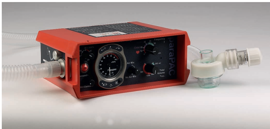
Figure 2.1 Pneupac® paraPAC. Reproduced with permission of Smiths Medical International.
