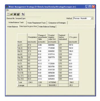
Fig. 6.10 Window for data input on water balance of the gross command area
