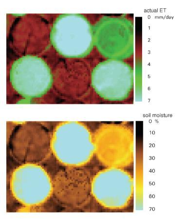
**Fig. 5.2** Irrespective of the level of technology used, the ET<sub>a</sub> and the soil moisture vary throughout the irrigated field. The images above show soil/moisture and ET<sub>a</sub> from center pivots, Washinton State, USA, Landsat 25 July, 2000. (courtesy WaterWatch, Wageningen).
