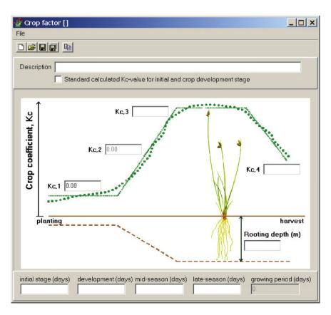
Fig. 6.8 Window for entering crop data (K<sub>c</sub>, growing period, rooting depth)
