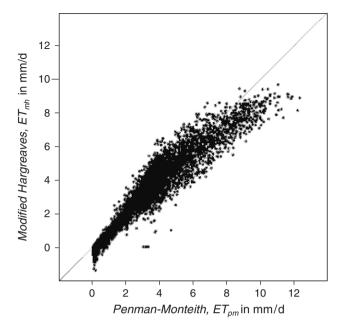
**Fig. 2.6** Scatter plot of the difference between monthly  $ET_0$  estimates using Penman-Monteith (PM) and modified Hargreaves-Samani (MH). A random 0.1% of the total points for each month are plotted (Droogers and Allen 2002)
