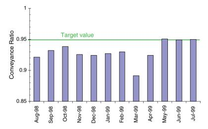
Fig. 5.11 Monthly values of the conveyance (outflow over inflow) ratio of the Nilo Coelho main canal (concrete lined, design capacity 20 m³/s, length 32.5 km)
