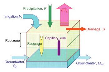
Fig. 1.7 Schematic water balance in an irrigated field (Bos 1984)
