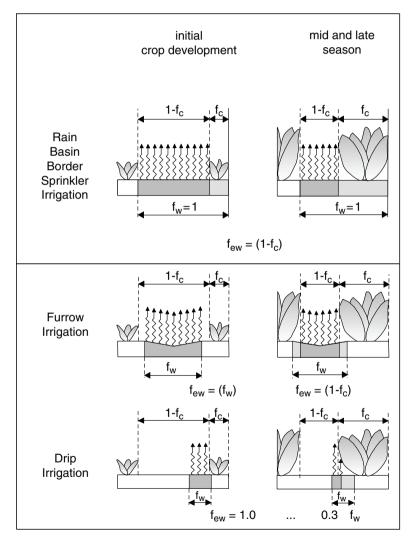
**Fig. 2.12** Crop determination of  $f_{ew}$  (greyed areas) as a function of the fraction of ground surface coverage  $(f_e)$  and the fraction of the surface wetted  $(f_w)$  (From Allen et al. 1998)
