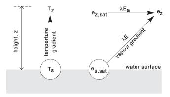
where the ratio  $c_p p_d/\lambda \epsilon$  is commonly replaced by  $\gamma$ , termed the psychrometric constant (kPa/°C). The problem with the above equations is that the surface temperature,  $T_s$ , is not generally known (not routinely measured). Penman therefore took three intermediate steps:
