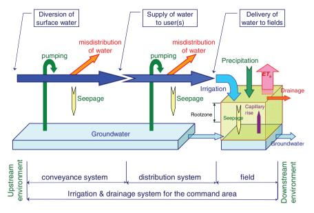
Fig. 1.9 Schematic flows of water within an irrigation and drainage system
