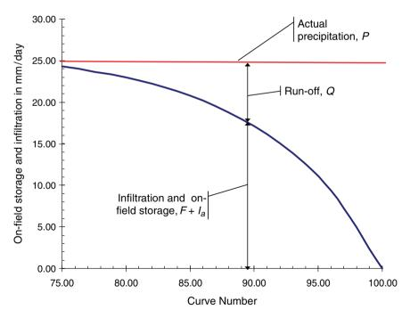
Fig. 3.8 Influence of the CN-value on the distribution between run-off and infiltration for a precipitation of  $25\,\mathrm{mm/day}$
