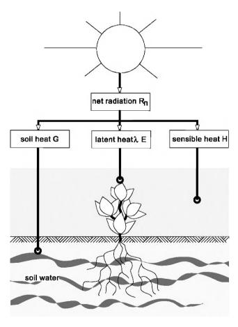
**Fig. 2.3** Illustrating the variables involved in the energy balance of the soil surface (Feddes and Lenselink 1994)
