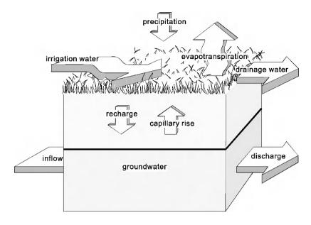
Fig. 4.1 The water balance of an irrigated field (Bos 1984)
