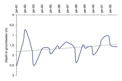
Fig. 4.6 Fluctuation of the depth to groundwater under an irrigated area
