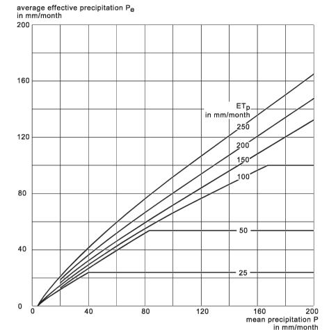
Fig. 3.3 Average monthly effective precipitation as related to the mean total monthly precipitation and the average monthly precipitation for a net irrigation application depth of 75 mm per turn
