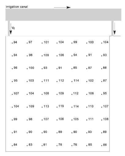
Fig. 5.3 Measured depths ( $V_{ail}$  in mm/turn) of irrigation water applied to a level basin (Till and Bos 1985)
