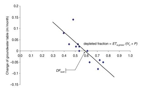
Fig. 4.7 Monthly change of groundwater table as a function of the depleted fraction, Nilo Coelho irrigated command area, Brazil (Bos 2004)
