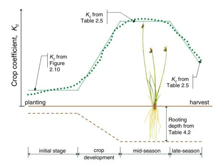
Fig. 2.9 FAO-style, linearized  $K_c$  curve with four crop stages and three  $K_c$  values relative to typical ground cover
