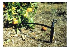
Sprinkler, downward fine spray. Multiple downward spraying nozzles reduce evaporation from 'rain drops' and increase uniformity (s < 0.1). These irrigation machines thus should (and can) operate at field application ratios (efficiencies) between 0.90% and 0.95%.
