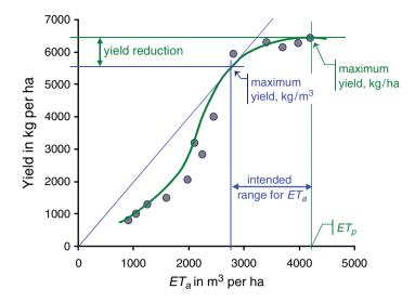
**Fig. 1.5** Crop production function showing the cumulative ET<sub>a</sub> versus yield for wheat, Central Great Plains, USA (Data points from Hanks et al. 1967)
