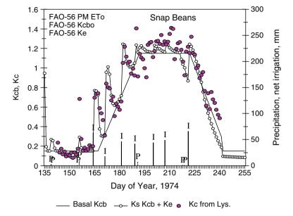
Fig. 2.13 Measured (circles) and estimated daily crop coefficients for a snap bean crop at Kimberly, Idaho. The basal crop curve ( $K_{cb}$ ) was derived from  $K_c$  values given in Table 2.5 (P = precipitation event and, I = irrigation (Data from J. Low Wright 1990))
