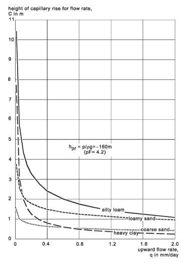
Fig. 4.4 Height of capillary rise as a function of the upward flow rate (flux) for four undisturbed Dutch soils
