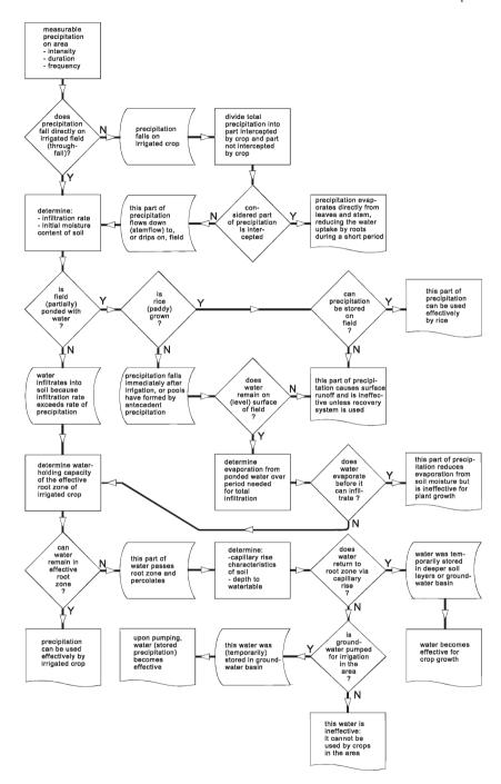
Fig. 3.2 Precipitation flow chart (Kopec et al. 1984)
