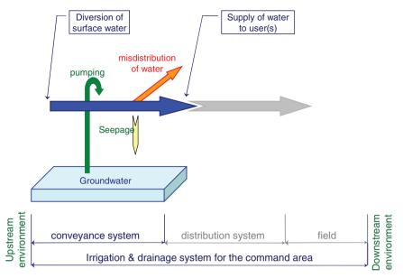
Fig. 5.9 The setting of the conveyance system
