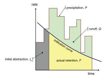
Fig. 3.4 The division of precipitation between initial abstraction, actual retention, and runoff
