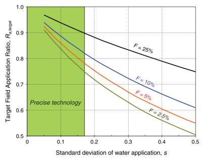
Fig. 5.4 Values of  $R_{a,target}$  as a function of the level of technology (the standard deviation of water application) and the part of the field that may receive less than the intended water need (F in percent of field)
