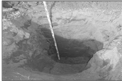
FIGURE 7.6 Soil excavation pit to obtain soil samples.
