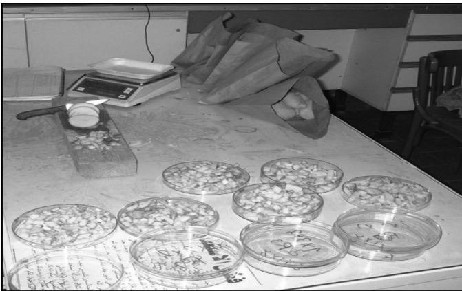
FIGURE 7.11 Cutting the tubers into small pieces for determination of dry matter content, specific density and total carbohydrates.
