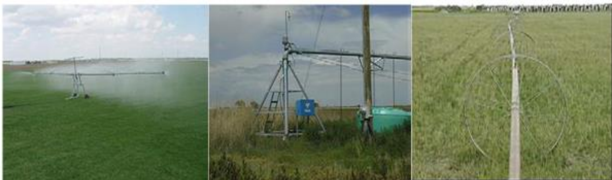
Fig. 36.1. Rotating type sprinkler irrigation systems.
