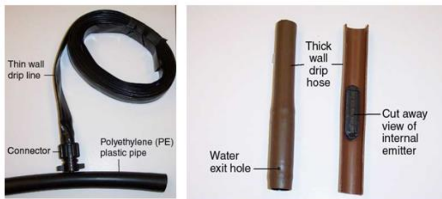
Fig. 42.11. Drip line with integrated emitters.
