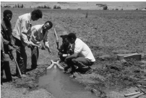
Fig. 5.35. Measuring the flow in a furrow using a portable flume.
