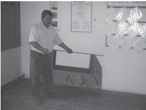
Fig. 5.33. (a) Portable sharp-crested rectangular weir for on-farm discharge measurement and (b) a typical location for flow measurement where the tertiary canal bifurcates.
