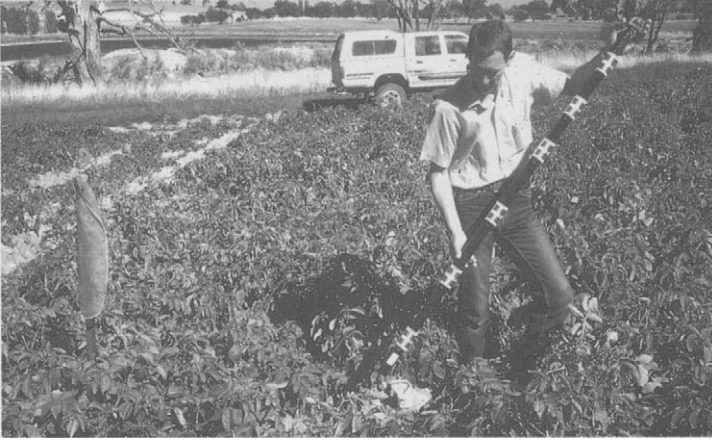
Figure 2.5 EnviroSCAN ® instrumentation removed from its access tube in potatoes
