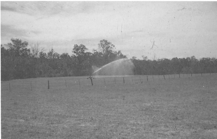
Figure 6.6 Typical spray pattern from a travelling irrigator, showing the substantial wetted width, and a good breakup of the spray across the width.
