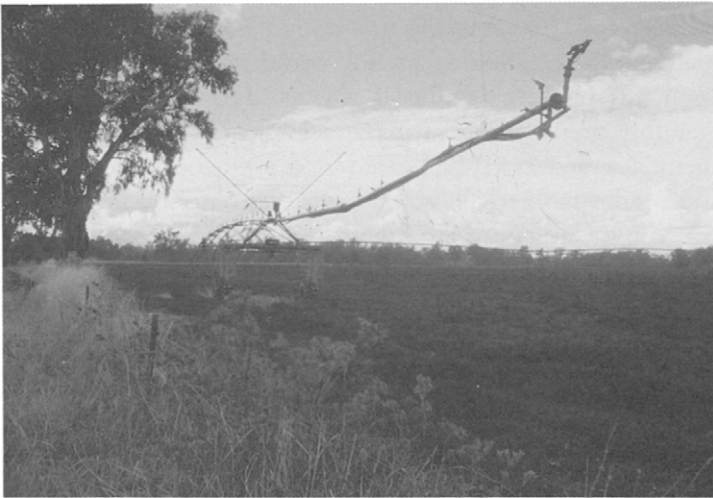
Figure 6.12 A corner watering extension is fitted to this centre-pivot machine. The last section of the sprayline can swing in and out to follow a non-circular boundary to the field.
