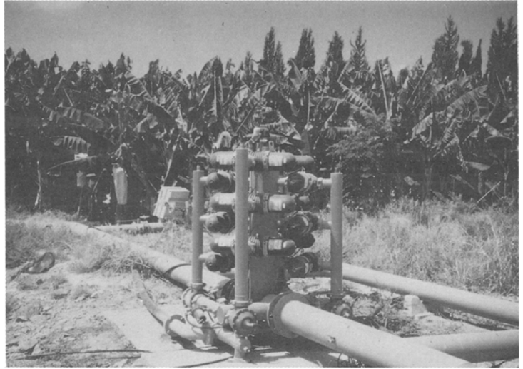
Figure 7.7 Multiple disc-type filters, mounted in a tower. This version is self-cleaning.
