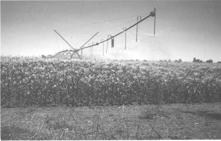
Figure 6.11 Drop tubes on this machine bring water closer to crop height, minimising wind disturbance, and enabling selection of low pressure nozzles.
