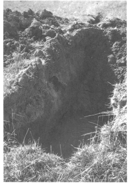
Figure 1.4 A series of test pits such as these can be used to inspect soil conditions throughout the depth of the profile. In this pit, note the light coloured silty material just below the topsoil, and heavy clay material in the subsoil. The water in the base of the pit may be caused by a high water table or by poor internal drainage
