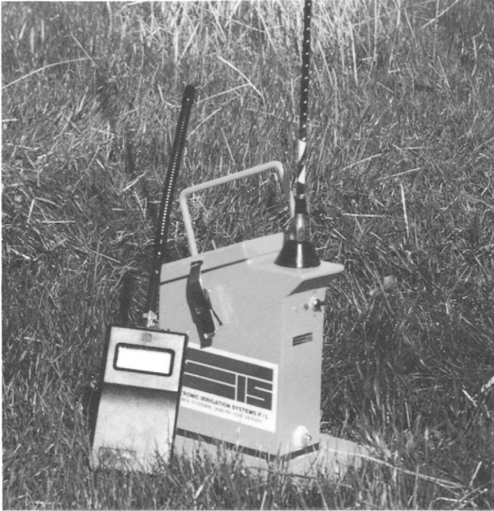
Figure 5.10 One type of sensor and its receiver to detect progress of the wetting front during irrigation. (Courtesy: Electronic Irrigation Systems P/L)
