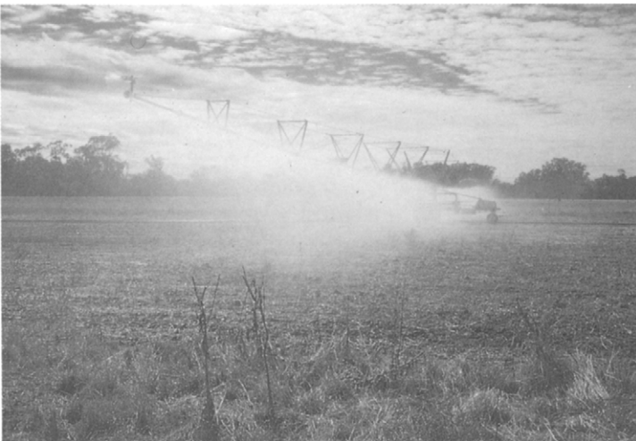
Figure 6.8 Low pressure boom type travelling irrigator
