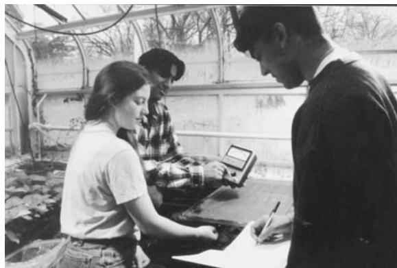
FIGURE 3.2 Photograph of students Ashish Goyan, Kathryn Timberlake, and Atul Rustgi measuring light intensity with a photo flux density meter (Ly-Cor, Inc.) in their shading experiment with seedlings of tree of joy, Camptotheca acuminata . (Photo courtesy of David Bay.)
