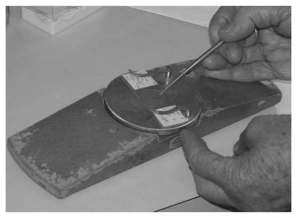
Fig. 3.5 Turntable for sealing cover slips on glass slides using a brush and insulating paint or other sealants.
