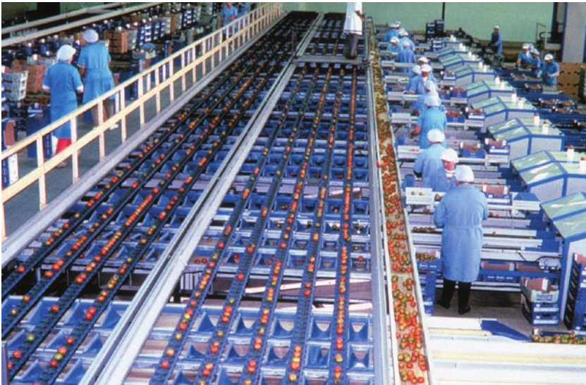
Photo 16.1. Classification and calibration are the basis of trade at a distance, without the physical presence of the commodities. The image shows a tomato classification machine.
