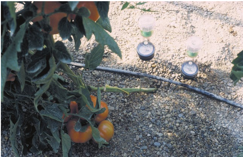
Photo 11.1. Tensiometers are increasingly used in greenhouses.
