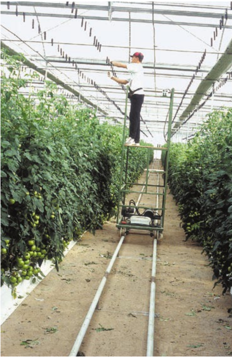
Photo 12.3. Use of rails (heating pipes) to move the lifting platform.
