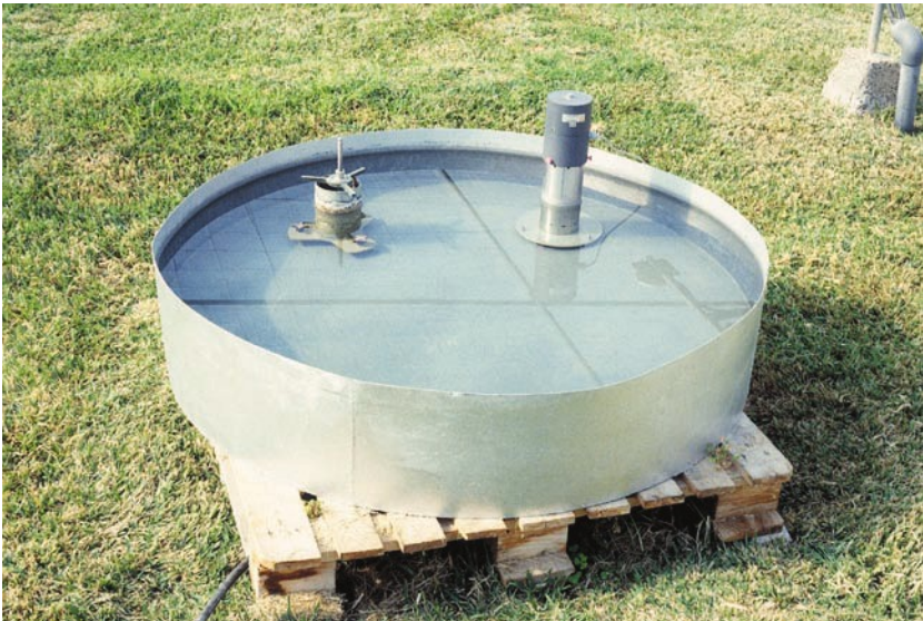
Photo 11.4. Class A evaporation pan.
