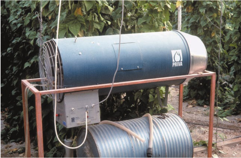
Photo 9.2. CO 2 generator that produces CO 2 by combustion.
