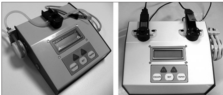
Figure 2. Pictures of the compact amperometric biosystem (single cell and two parallel cells model) that integrates biologic material sample holder and measurement chamber with electronics and automatic fluidic. The instrument is produced by the company Biosensor Srl (Palombara Sabina-Rome, Italy).
