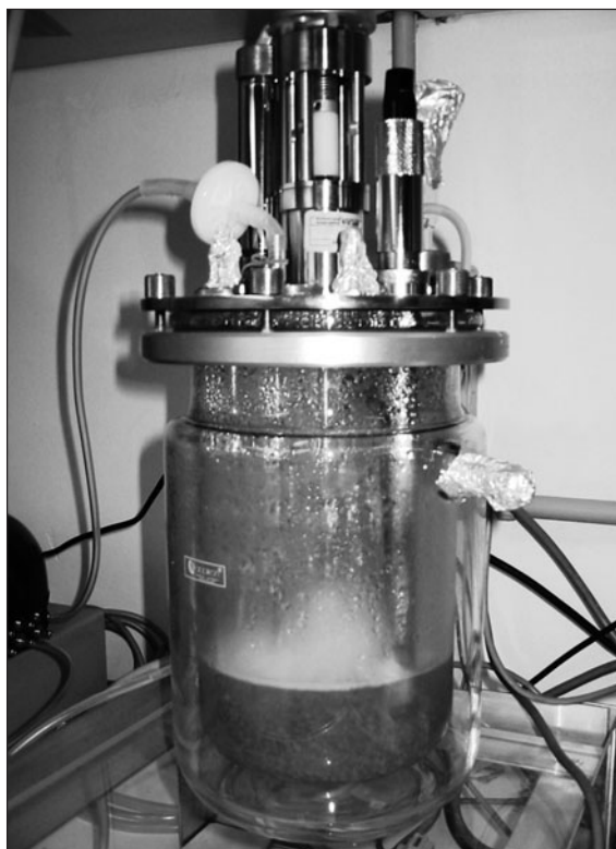
Figure 1. Scale up of Salvia cinnabarina hairy root culture in bioreactor (Applikon®, Germany).
