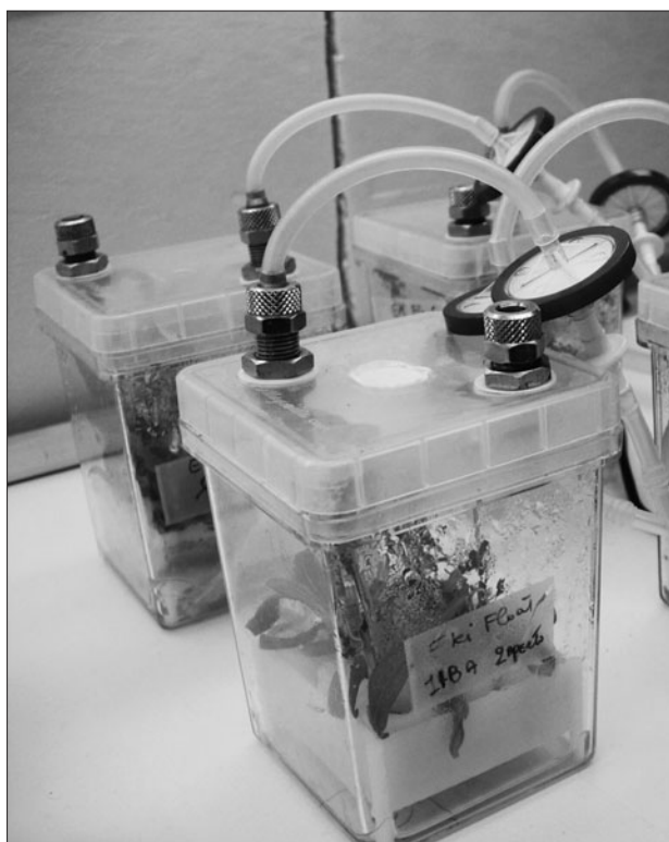
Figure 6. Microfloating system: a pump inflates air into the vessels under the liquid medium trough flexible silicon pipes.
