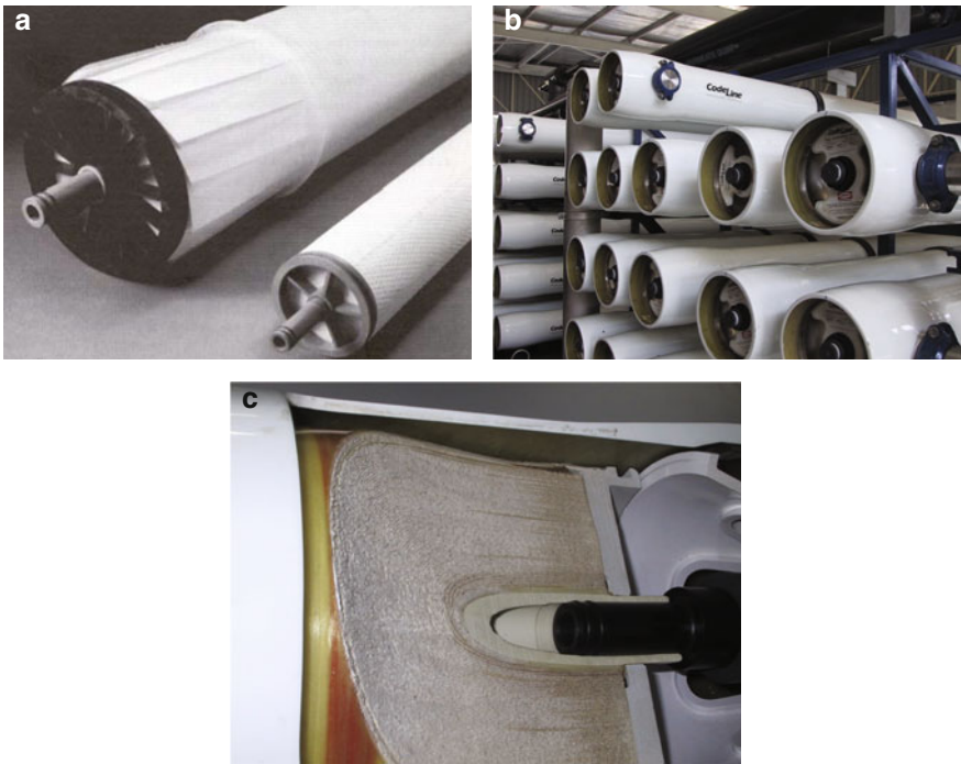
Fig. 7.11. Industrial-scale spiral-wound modules.
