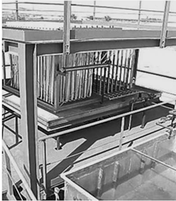
Fig. 6 An illustration of the WAIV technology. (Obtained from J. Gilron, Y. Folkman, R. Savliev, M. Waisman, O. Kedem, WAIV – wind aided intensified evaporation for reduction of desalination brine volume, Desalination 158 (2003) 205–214, http://dx.doi.org/10.1016/S0011-9164(03)00453-3 ).
