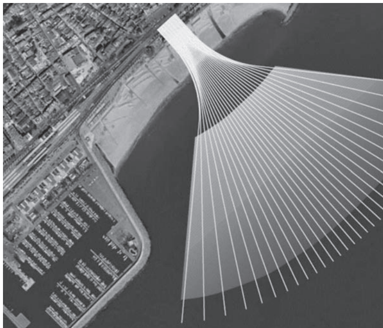
FIGURE 6.11 HDD intake of San Pedro del Pinatar SWRO plant.
