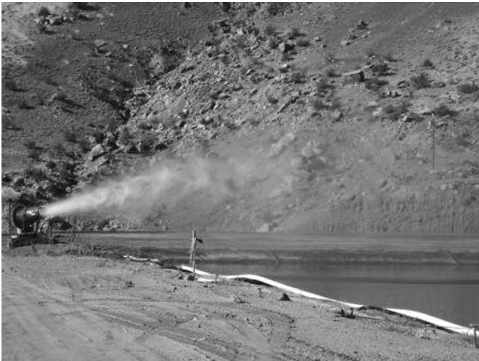
FIGURE 16.40 Spray evaporation pond.
