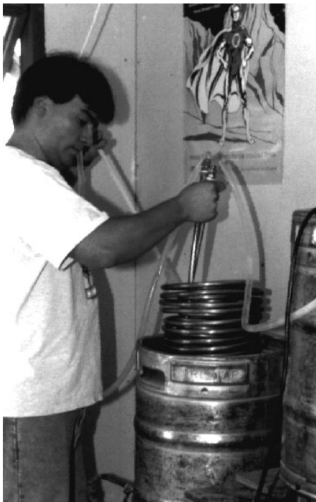
Figure 105: Now the boil is over and its time to chill the wort. Joe Brewer uses a large immersion wort chiller to chill the 6 gallons of wort.
