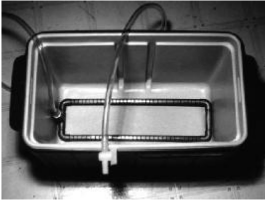
Figure 92: This view shows the slots cut in the copper manifold. The design of copper manifolds is discussed in Appendix D.
