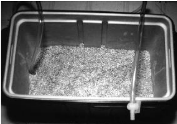
Figure 93: The lautering manifold is now installed in the bottom of the cooler. Designs will vary depending on what you have to work with.
