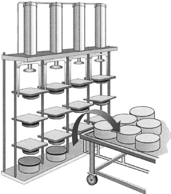
Figure 10 Vertical pressing unit with pneumatically operated pressing plates. (From Ref. 1, courtesy of Tetra Pak Processing Systems AB, Sweden.)
