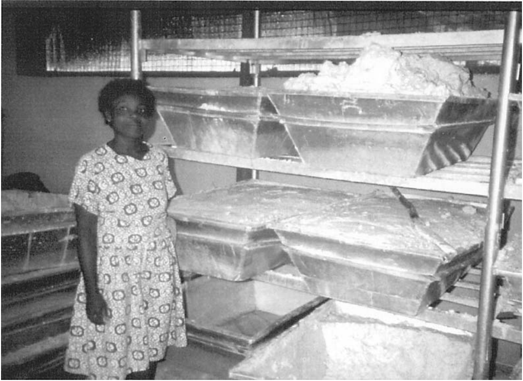
Figure 3 An upgraded site for maize fermentation. The figure shows the fermentors made of aluminum.
