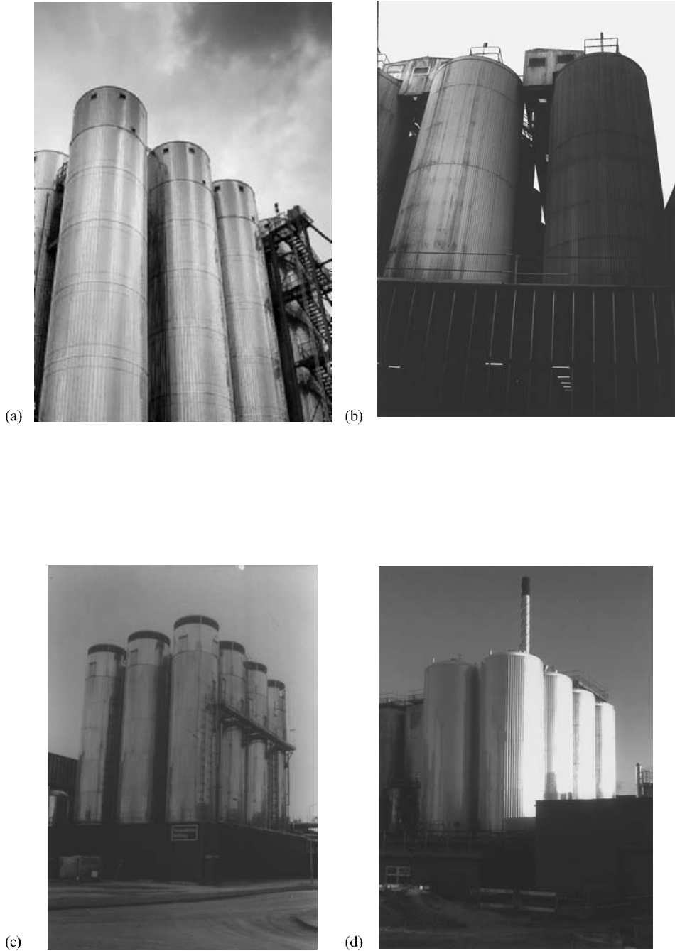
Fig. 5.12 Cylindeconical fermenters (a) courtesy of Briggs PLC, (b) kindly supplied by Maxine Bellfield of Vaux Breweries, (c) kindly supplied by Harry White, Bass Brewers and (d) courtesy of Ian Dobbs, Bass Brewers.
