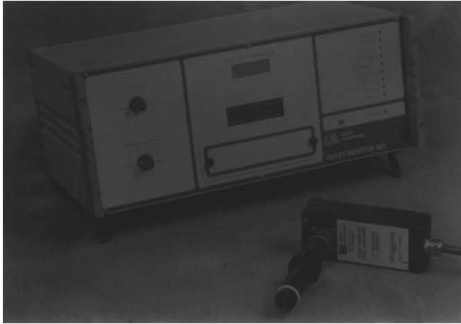
Fig. 6.9 Biomass meter (courtesy of Aber Instruments).
