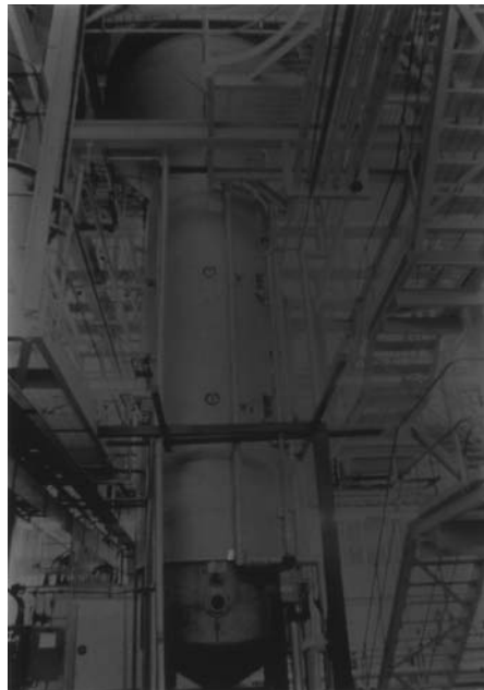
Fig. 5.41 Tower fermenter (kindly supplied by Harry White, Bass Brewers).
