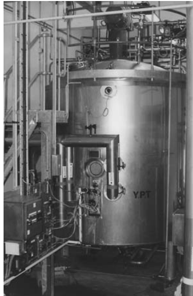
Fig. 6.30 Yeast oxygenation plant (courtesy of Bass Brewers Limited).
