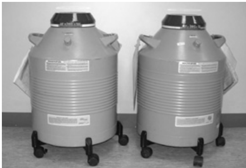
Fig. 7.2 Liquid nitrogen storage cryovessals (Kindly supplied by Steph Valenti of Bass Brewers).
