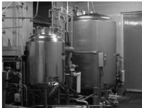
Fig. 7.5 Conventional yeast propagator (kindly supplied by Mark Grey and Peter Smith, Bass Brewers).
