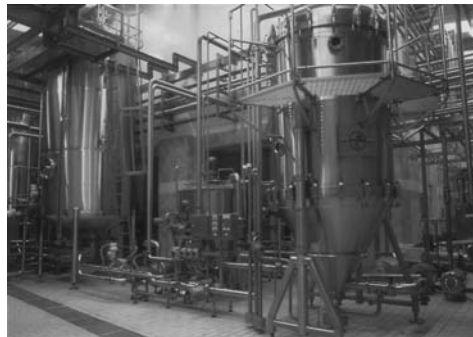
Fig. 2.13 Candle filter (kindly provided by Steve Freckleton, Bass Brewers).
