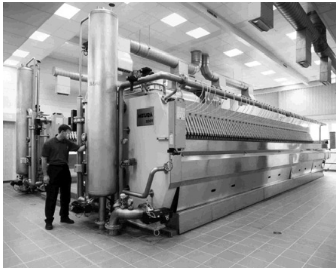
Fig. 2.9 Mash filter (kindly provided by Meura Ltd).
