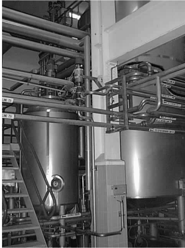
Fig. 7.8 Two-tank aerobic propagation system at Bass Brewers Limited, Alton Brewery (kindly supplied by Jim Appelbee, Bass Brewers).
