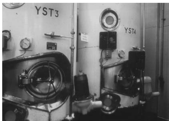
Fig. 7.13 Vessel for storage of pitching yeast slurry (kindly supplied by (a) Steph Valente, Bass Brewers and (b), (c) Ian Dobbs, Bass Brewers).
