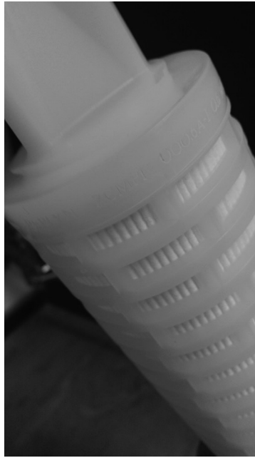
Figure 11.3 A cartridge filter showing the pleated membrane and support structure. This is contained in a stainless steel housing and filtration is from outside to inside this unit.
