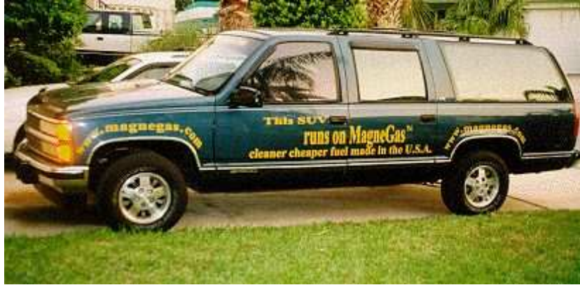
Figure 10.16. A picture of a Chevrolet Suburban SUV 1992 converted by the author to operate as a bifuel gasoline/magnegas with a switch on the dashboard permitting to pass from one fuel to the other while driving. Bifuel cars are produced by numerous carmakers to operate on gasoline and natural gas. The same cars can operate on magnegas (in place of natural gas) with the sole adjustment of the pressure regulator to optimize the stoichiometric ratio air/fuel, since the latter for magnegas is much smaller than that for natural gas because magnegas is very rich internally in oxygen, thus requiring a fraction of the air needed by natural gas to operate. These bifuel cars are ideally suited for the magnegas technology because, when magnegas runs out, one can still reach the magnegas refilling station on gasoline (see website [5b] for details).
