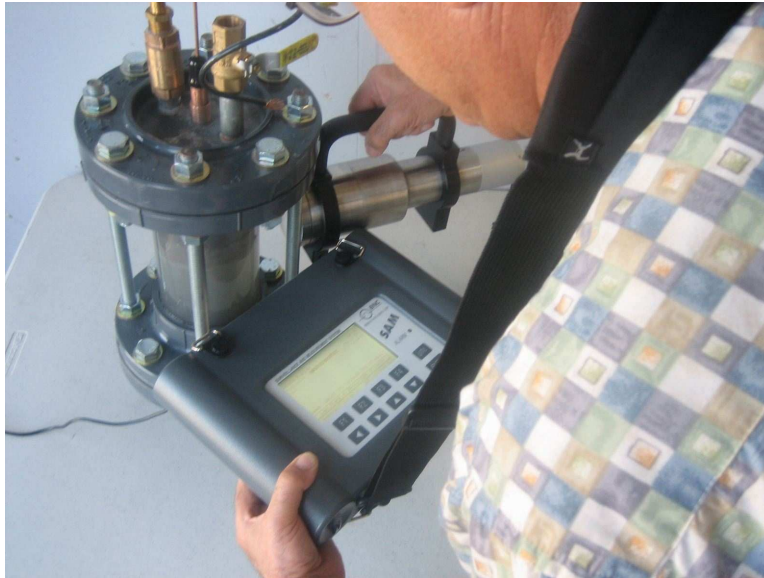
Figure 6.28. A picture of Klystron I and of detector SAM 935. Note the similarity with the klystron used in tests [116,117], but also the primary differences being given by the use of metal walls for tests [116,117], and transparent polycarbonate walls for tests [118,119]. The latter were selected so as to permit the visual identification of the creation of an interior electric arc with a gap between the electrodes, the latter being necessary to assure the creation of a discharge through the hydrogen gas.
