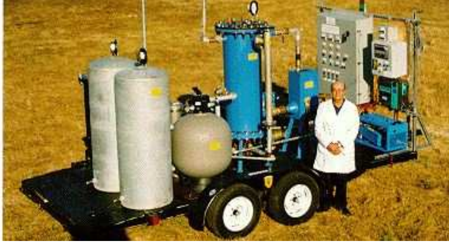
Figure 10.14. Picture of a 50 Kw Santilli's Hadronic Reactor (PlasmaArcFlow Recycler) mounted on a trailer for mobility to conduct test recycling where liquid wastes are located. This recycler can produce up to 84,000 scf (up to 2.4M liters) of magnegas per week corresponding to about 560 gasoline gallon equivalent (2,100 gasoline liter equivalent) of magnegas per week (see website [5b] for details).
