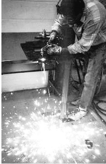
Figure 10.33. A view of metal cutting via magnegas. Independent certifications by various users have established that: 1) magnegas has a pre-heat time at least half that by acetylene (which is currently used for metal cutting and has an energy content of 2,300 BTU/cf); 2) magnegas cuts metal at least 50% faster than acetylene; 3) the cut produced by magnegas is much smoother without edges as compared to that by acetylene; 4) magnegas exhaust does not contain carcinogenic or other toxic substances, while that of acetylene is perhaps the most carcinogenic and toxic of all fuels; 5) magnegas cutting does not produce the "flash-back" (local explosion of paint over metal) typical of acetylene; 6) magnegas is dramatically safer than acetylene, which is unstable and one of the most dangerous fuels currently used; and 7) magnegas cost about 1/2 that of acetylene.
