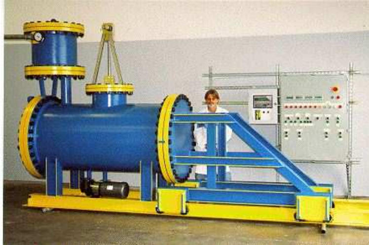
Figure 10.13. Picture of a 250 Kw Santilli's Hadronic Reactor (also called PlasmaArcFlow Reactor) with the panels of its completely automatic and remote controls, to recycle liquid waste into magnegas usable for any fuel application, a large amount of heat and carbonaceous precipitates used to produce the electrodes. This Reactor can produce up to 5000,000 scf (140 millions liters) of magnegas per week of 24 hours work per day corresponding to 3,000 gasoline gallon equivalent (11,000 gasoline liter equivalent) of magnegas per week computed on the basis that: 1) Gasoline contains about 110,000 BTU/g (about 29,000 BTU/liter); 2) Magnegas has the low energy content of 750 BTU/scf (26 BTU/liter); and 3) the "gasoline gallon equivalent" is given by about 150 scf of magnegas ("gasoline liter equivalent" is given by about 29 liters of magnegas). PlasmaArcFlow reactors are completely self-contained. Consequently, they release no solid, liquid or gas to the environment and cause no noise or odor pollution (see website [5b] for details).
